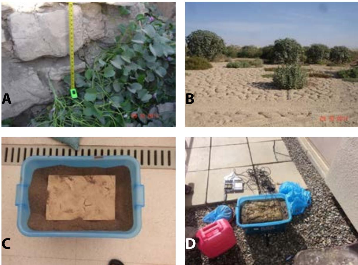
**Figure 1.** Smart block-fracture structure in the field and experimental replicate: (A) Silt blocks in a pedon dug in the reservoir area of the Al-Khod dam (left panel); (B) surface view of the site (right panel), (C) Silt block (light colour) collected from the reservoir and trimmed to fit the blue plastic box. Sheaths of loose sand (proppant) have darker colour, and (D) Measurements of VMC-temperature after the first ponding.
