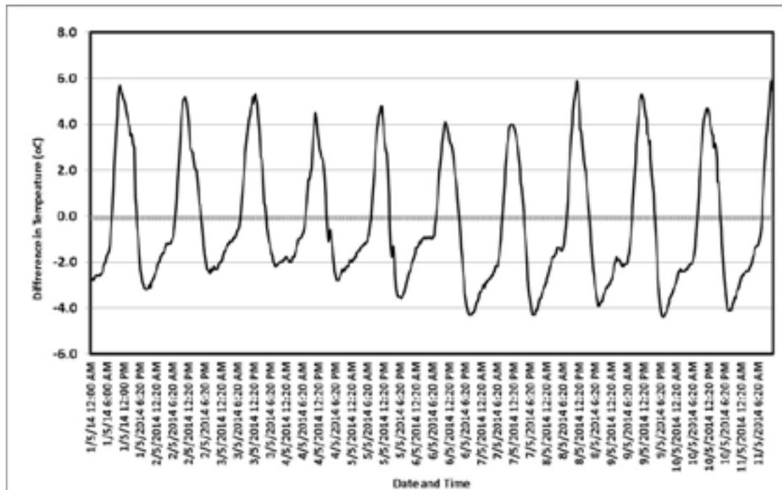
**Figure 4.** Difference in temperature ( $^{\circ}\text{C}$ ) between the sheath and the centre of the block for selected period between 1/5/2014 12:00 pm and 11/5/2014 12:00 am (after re-wetting).
