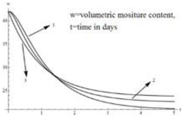
Figure 6. Modelled VMC as a function of time (in days) at the middle of the block.
