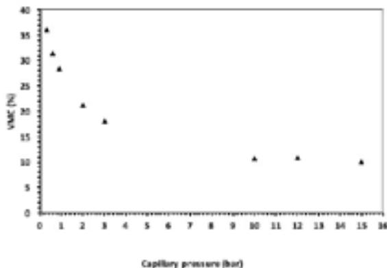
Figure 5. Water retention curve of block soil.
