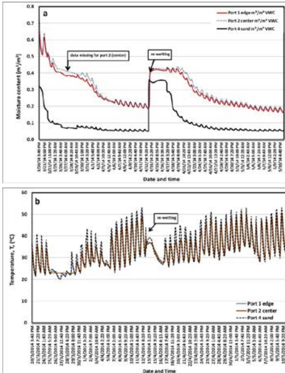
**Figure 3.** VMC (a) and temperature (b) as a function of time during the imbibition-desiccation experiment.
