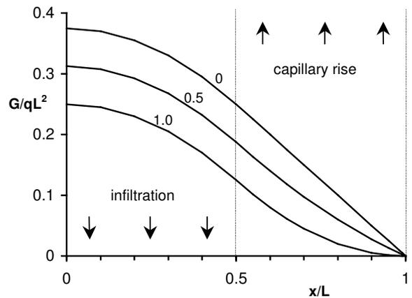
Figure 4. The variation of  $G/qL^2$  with  $x/L$  or  $L' = 0.5$  for three values of  $e/q$  shown by the curves.
