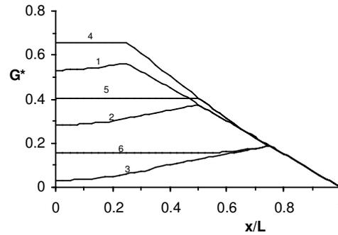
Figure 7. The variation of  $G^* = G_{av}/eL^2$  with  $x/L$  when water is injected into wells at  $x = L_a$  at a rate  $Q_i$  and there is capillary rise with loss of water due to evaporation at a rate  $e$  between  $L' < x < L''$ . Curves 1, 2 and 3,  $L'/L = 0$ ,  $L''/L = 0.5$ ; curves 4, 5 and 6,  $L'/L = 0.5$ ,  $L''/L = 1.0$ ; curves 1 and 4,  $L_i = 0.25$ ; curves 2 and 5,  $L_i = 0.5$ ; and curves 3 and 6,  $L_i = 0.75$ ;  $Q_i/BL_e = 1.0$ .
