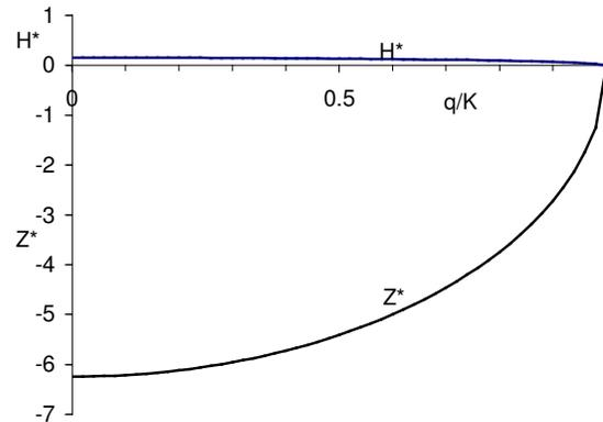
**Figure 3.** The Dupuit-Forchheimer estimate of the fresh-water lens with uniform steady infiltration, shown as  $H^* = (H/L)\sqrt{(K/q)}$  and  $Z^* = (Z/L)\sqrt{(K/q)}$  as functions of  $x/L$ .
