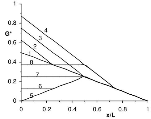
Figure 5. The variation of  $G^* = G_{av}B/Q_iL$  with  $x/L$  when there are injection wells at  $x = L_i$  and abstraction wells at  $x = L_a$  for  $Q_a/Q_i = 0.5$ . Curves 1, 2, 3 and 4,  $L_i/L = 0$ ; curves 5, 6, 7 and 8,  $L_i/L = 0.5$ ; curves 1 and 5,  $L_a/L = 0$ ; curves 2 and 6,  $L_a/L = 0.25$ ; curves 3 and 7,  $L_a/L = 0.5$ ; and curves 4 and 8,  $L_a/L = 0.75$ .
