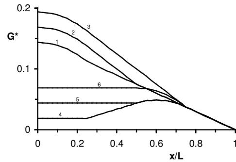
Figure 6. The variation of  $G^* = G_{av}/qL^2$  with  $x/L$  when there is infiltration at a rate  $q$  on to a surface strip  $L' < x < L''$  and abstraction from wells at  $x = L_a$  at a rate  $Q_a$ . Curves 1, 2 and 3,  $L'/L = 0$ ,  $L''/L = 0.5$ ; curves 4, 5 and 6,  $L'/L = 0.5$ ,  $L''/L = 1.0$ ; curves 1 and 4,  $L_a = 0.25$ ; curves 2 and 5,  $L_a = 0.5$ ; and curves 3 and 6,  $L_a = 0.75$ ;  $Q_a/BL_q = 0.1$ .
