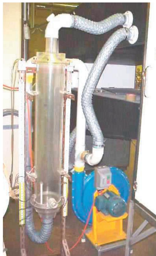
Figure 1. Fluidised bed drying experimental setup.
