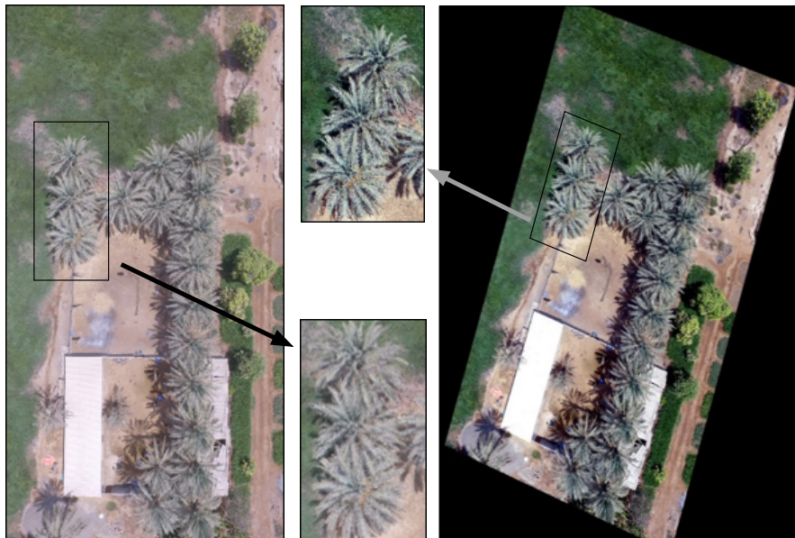
Figure 7. Orthorectification process of site number 2
