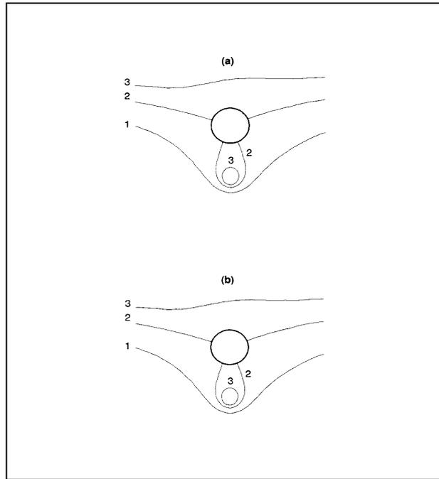
**Figure 8 (a, b).** The numerically obtained streamlines,  $\Psi$ , for  $\beta = 1.5$  with a mesh size  $40 \times 160$ . The streamlines labelled 1, 2 and 3 correspond to  $\Psi = -1, 0$  and  $0.7$ , respectively.
