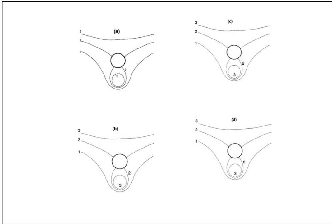
**Figure 6 (a,b,c, d).** The numerically obtained streamlines,  $\Psi$ , for  $\beta = 3$  with a mesh size  $40 \times 160$ . The streamlines labelled 1, 2 and 3 correspond to  $\Psi = -1, 0$  and  $0.7$ , respectively.
