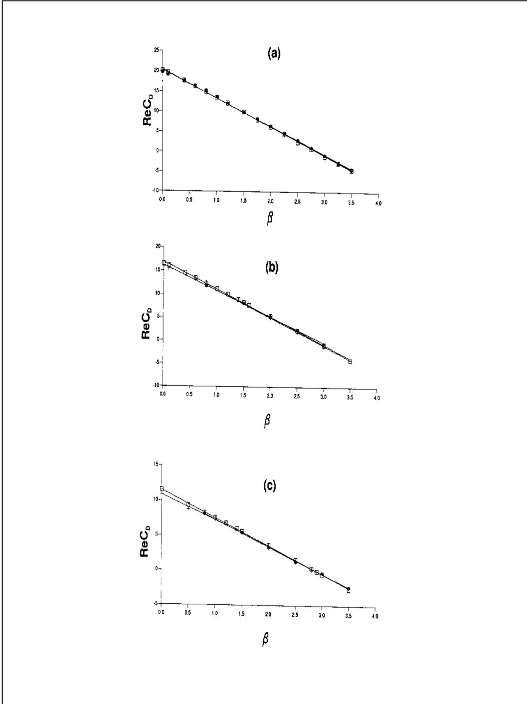
**Figure 3.** The variation of  $\text{Re} C_D$  as a function of  $\beta$   $\diamond\diamond\diamond 10 \times 40, ++ + 20 \times 80, *** 40 \times 160$ .
