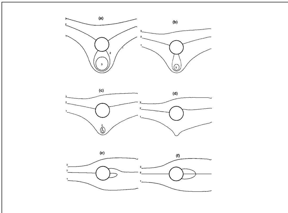
**Figure 10 (a, b, c, d, e, f).** The numerically obtained streamlines,  $\Psi$ , for  $Re = 20$  with a mesh size  $40 \times 160$ . The streamlines labelled 1, 2 and 3 correspond to  $\Psi = -1, 0$  and  $0.7$ , respectively. (a)  $\beta = 3$ , (b)  $\beta = 1.5$ , (c)  $\beta = 1$ , (d)  $\beta = 0.5$ , (e)  $\beta = 0.1$ , and (f)  $\beta = 0$ .
