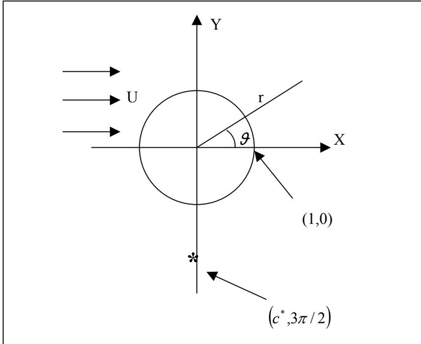
**Figure 1.** The geometry of the circular cylinder and the position of the rotlet
