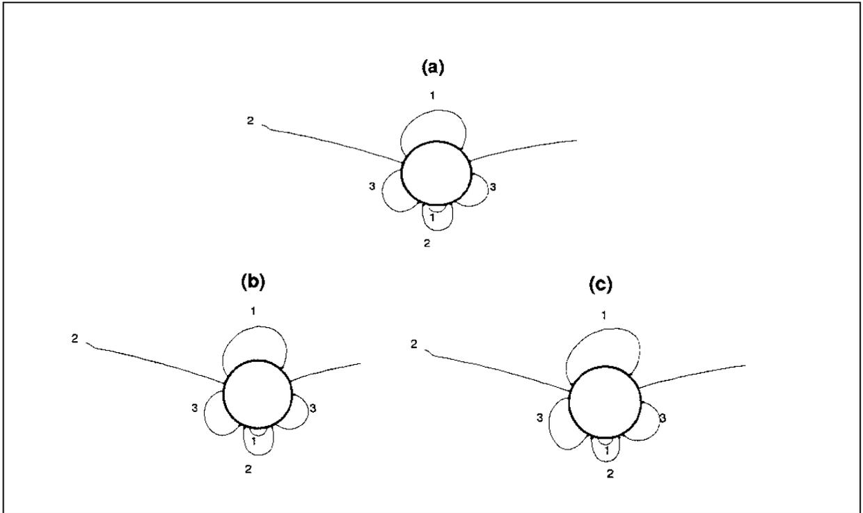
**Figure 9 (a, b, c).** The numerically obtained vorticity,  $\omega$ , for  $\beta = 1.5$  with a mesh size  $40 \times 160$ . The streamlines labelled 1, 2 and 3 correspond to  $\omega = -0.4, 0$  and  $0.4$ , respectively.
