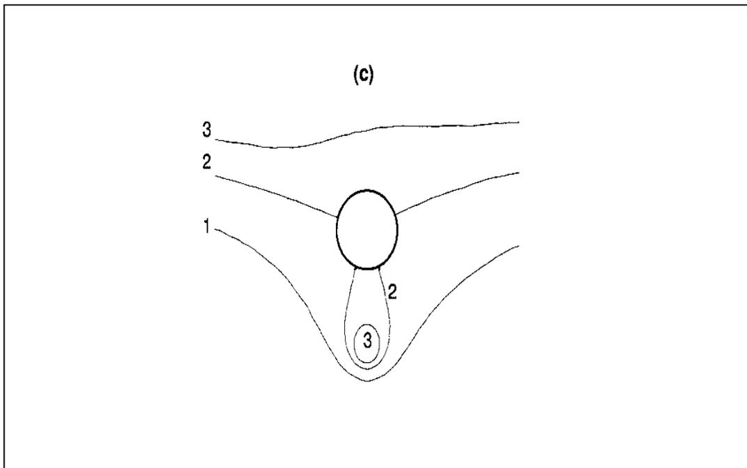
**Figure 8 (c).** The numerically obtained streamlines,  $\Psi$ , for  $\beta = 1.5$  with a mesh size  $40 \times 160$ . The streamlines labelled 1, 2 and 3 correspond to  $\Psi = -1, 0$  and  $0.7$ , respectively. (a)  $Re = 1$ , (b)  $Re = 3$ , (c)  $Re = 5$ .
