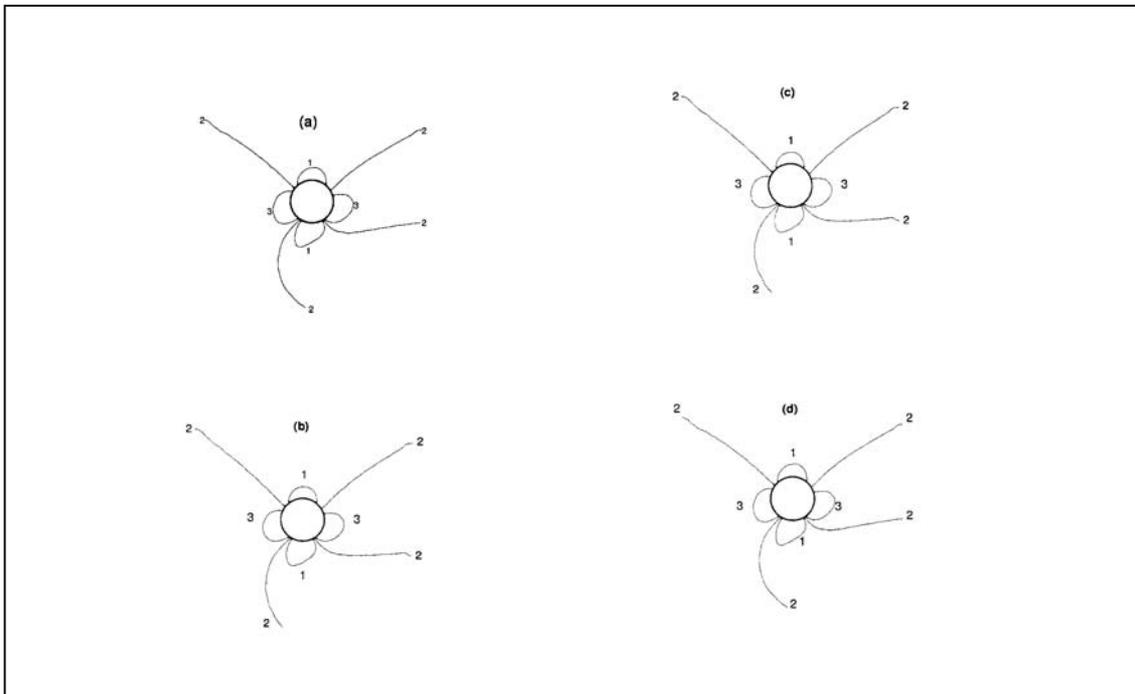
**Figure 7(a, b, c, d).** The numerically obtained vorticity,  $\omega$ , for  $\beta = 3$  with a mesh size  $40 \times 160$ . The streamlines labelled 1, 2 and 3 correspond to  $\omega = -0.4, 0$  and  $0.4$ , respectively.
