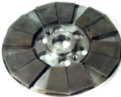
Figure 15. Six-pole inner rotor for 2.5 kW experimental machine.
