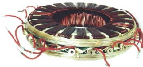
Figure 13. Toroidal stator with 11-phase winding.
