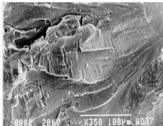
**Figure 10.** Fracture surface in Al- Alloy, aged for 6 h at 560 K.
