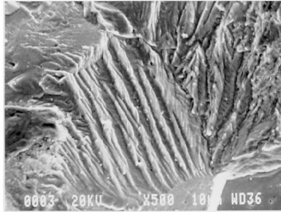
**Figure 8.** Cleavage fracture with fatigue striations, aged for 5 h at 480 K.
