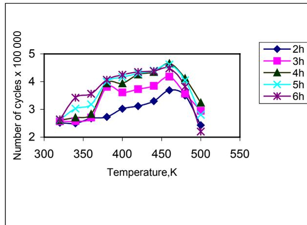
**Figure 2.** Effect of aging temperature at constant time on fatigue resistance properties of 6063 A-A.
