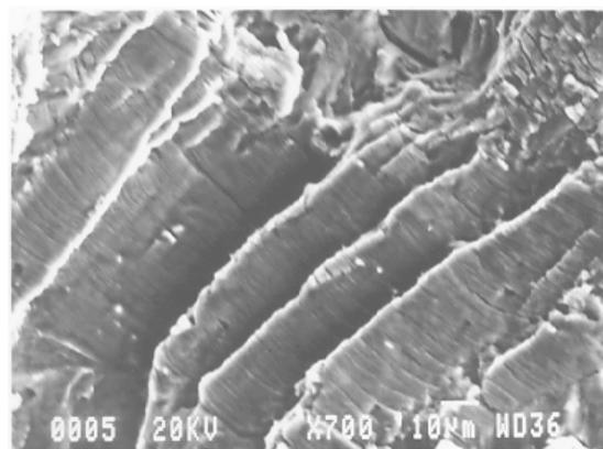
**Figure 7.** Fatigue striations in 6063 Al-Alloy, aged for 3 h at 370 K.
