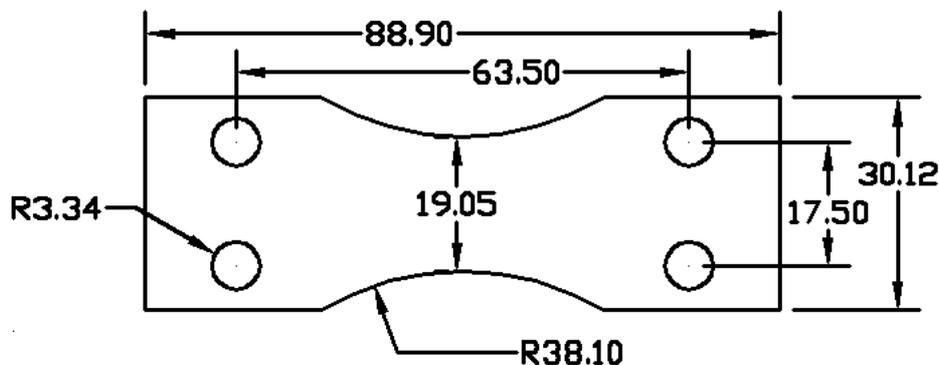
**Figure 1.** Standard fatigue specimen according to BS3518 specification in mm.
