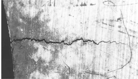
**Figure 5.** Crack initiation and propagation in 6063 Al-Alloy, aged for 3 h at 350 K.
