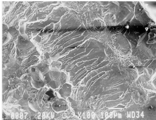
**Figure 9.** Cleavage fracture, aged for 5 h at 480 K.
