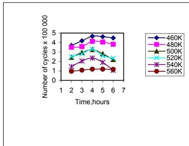
**Figure 4.** Effect of aging time at constant temperature (460-560 K) on fatigue resistance properties of 6063 A-A.
