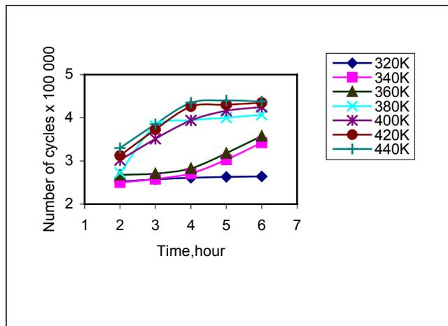
**Figure 3.** Effect of aging time at constant temperature (320-440 K) on fatigue resistance properties of 6063 A-A.
