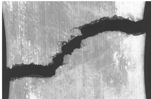
**Figure 6.** Fracture surface of 6063 Al-Alloy, aged for 5 h at 460 K.
