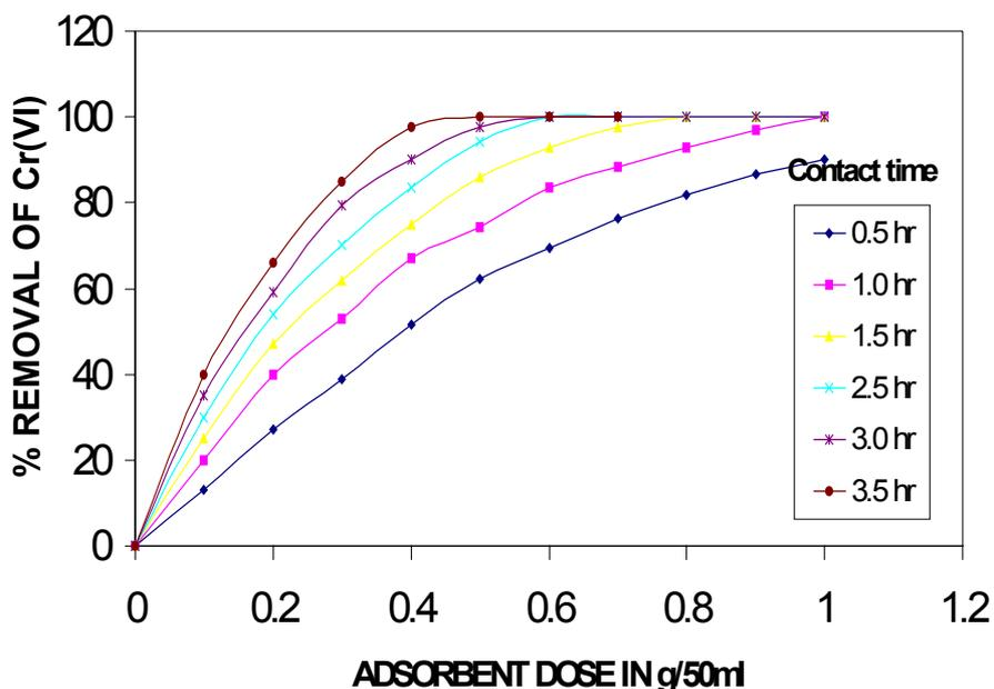
Figure 2. Effects of adsorbent dose at different contact time on Cr (VI) removal.
