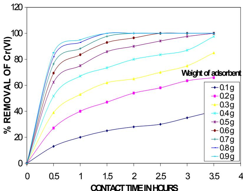
Figure 1. Effects of contact time at different adsorbent (bagasse) doses on Cr (VI) removal.
