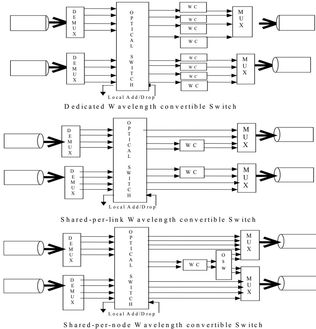
**Figure 2.** Wavelength-convertible switch architecture alternatives.
