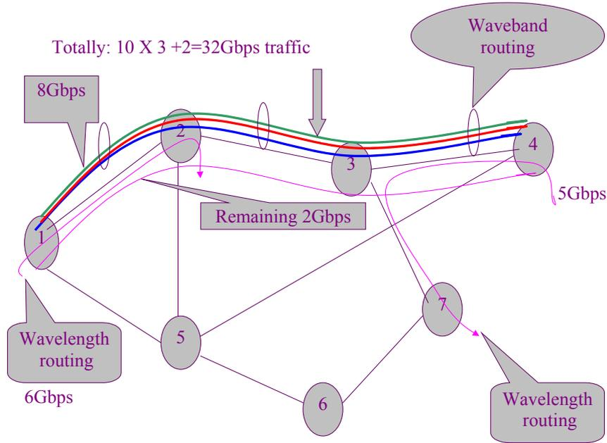
**Figure 4.** Hybrid waveband and wavelength routing.
