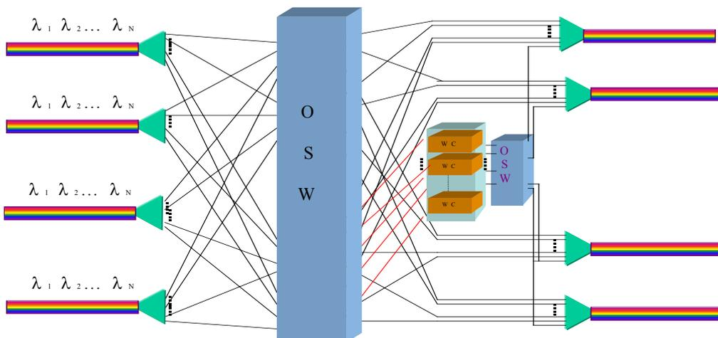
Figure 3. X% Wavelength-convertible switch architecture.
