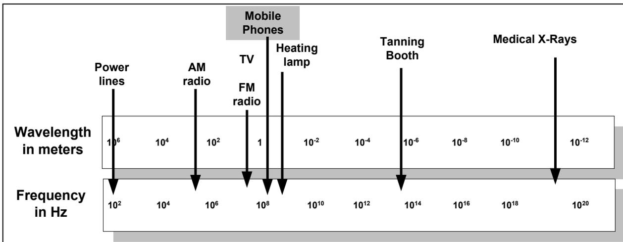
**Figure 1.** Mobile phone position in electromagnetic spectrum.
