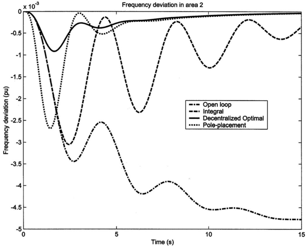
Figure 6. Area 2 dynamic response under a sudden load change in area 1.
