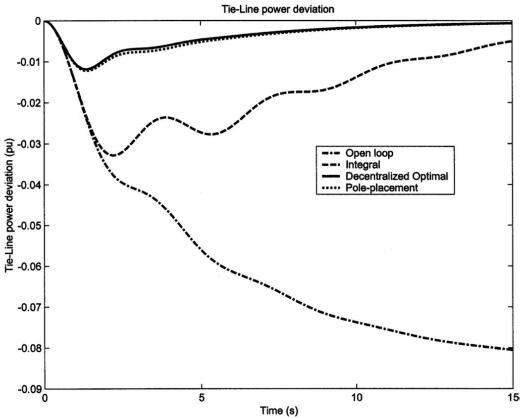
Figure 7. Tie-line dynamic response after a sudden load change in area 1.
