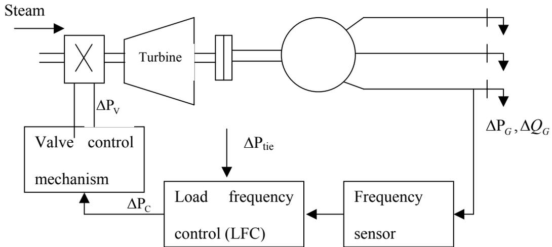
**Figure 1.** Schematic diagram of LFC and AVR of a generator.
