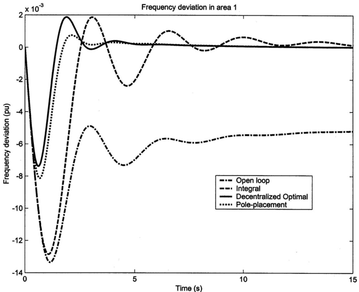
**Figure 5.** Area 1 dynamic response under a sudden load change in area 1.
