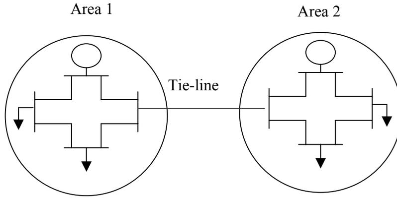
**Figure 2.** Single-line diagram of two-area.
