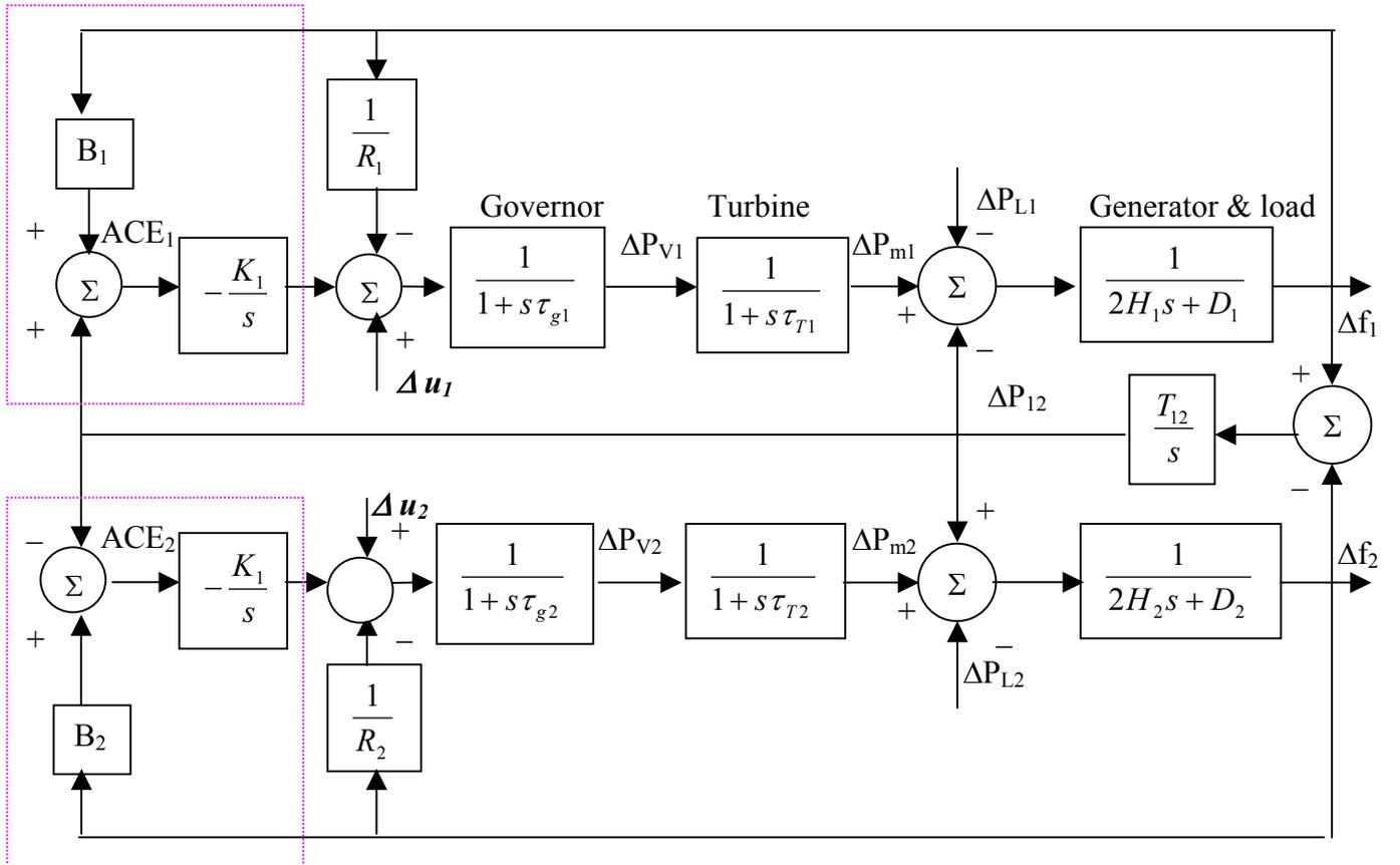
Figure 3. Block diagram of load frequency control (LFC) of two-area.
