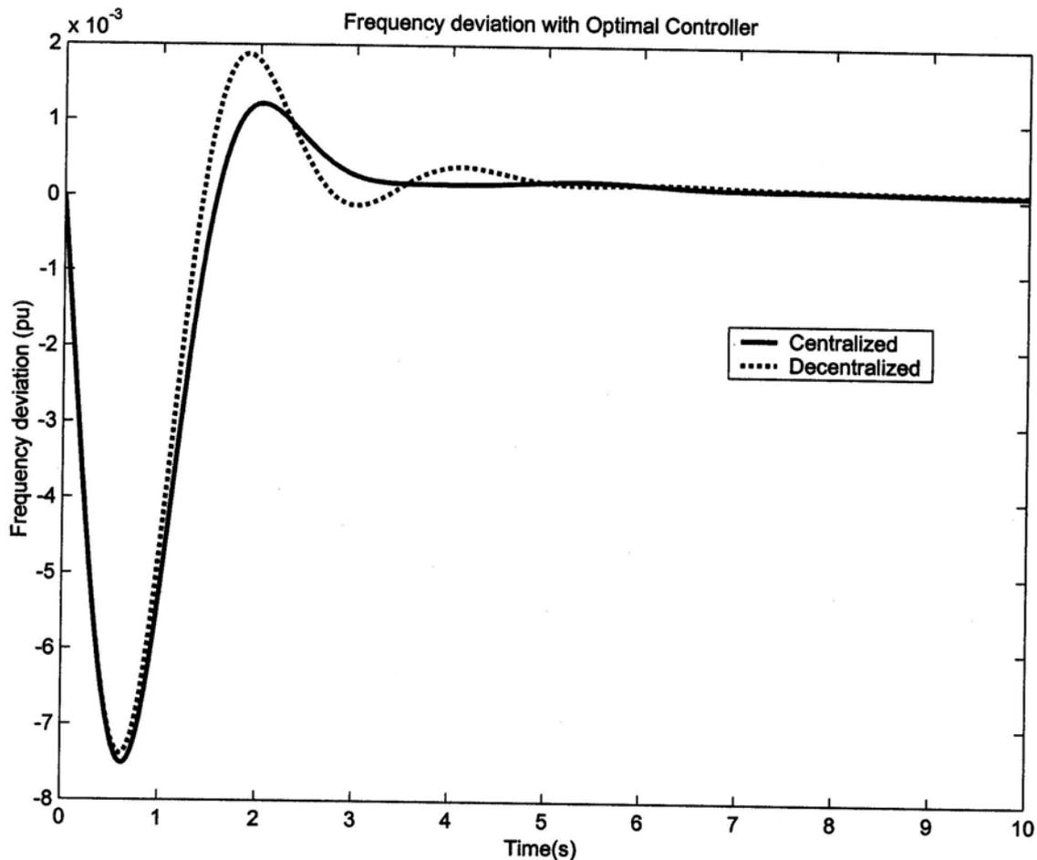
**Figure 4.** System dynamic response with centralized / decentralized optimal controller.
