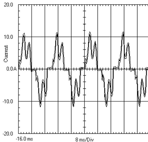
**Figure 8.** VSD line current fed from a distorted supply.
