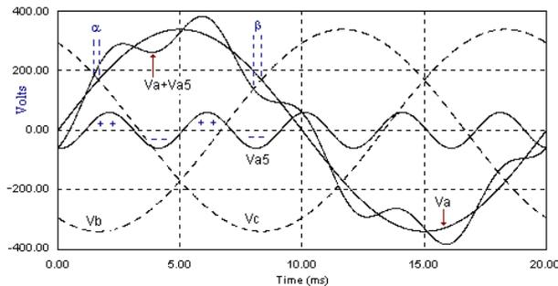
**Figure 4.** Effect of 5<sup>th</sup> harmonic voltage on rectifier current conduction angle. (note: scale for 5<sup>th</sup> harmonic current is greatly magnified).
