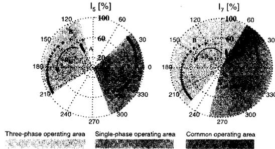
**Figure 9.** Polar plots for 5<sup>th</sup> and 7<sup>th</sup> harmonics for various short circuit ratios and argument of short circuit impedance equal to 80<sup>0</sup>.
