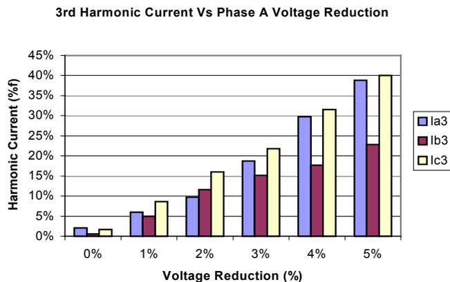
**Figure 5.** Effect on 3<sup>rd</sup> harmonic current with varying A-phase voltage.
