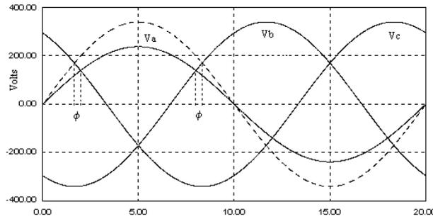
**Figure 3.** Effect of current conduction period with a change in voltage level.
