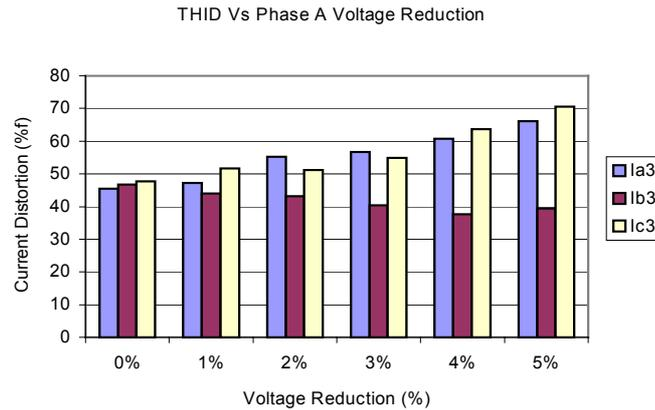
**Figure 6.** Effect on total harmonic current distortion with varying phase A voltage.
