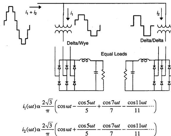
**Figure 10.** Two separate six pulse rectifier currents combine to a twelve pulse rectifier current.
