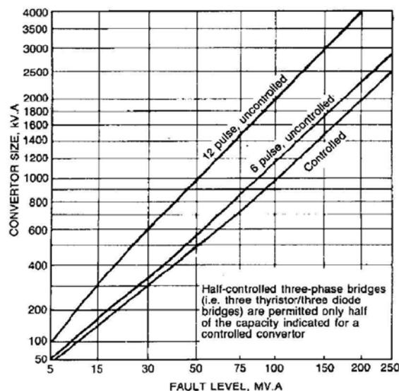
Figure 12. Equipment size in stage 3 (AS 2279).
