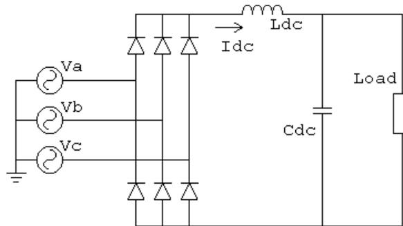
**Figure 1.** Complete circuit diagram of the 6-pulse rectifier.
