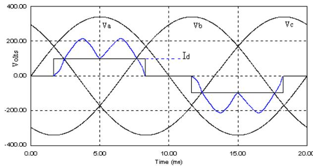
**Figure 2.** Theoretical representation of line current for an ideal 6-pulse rectifier.
