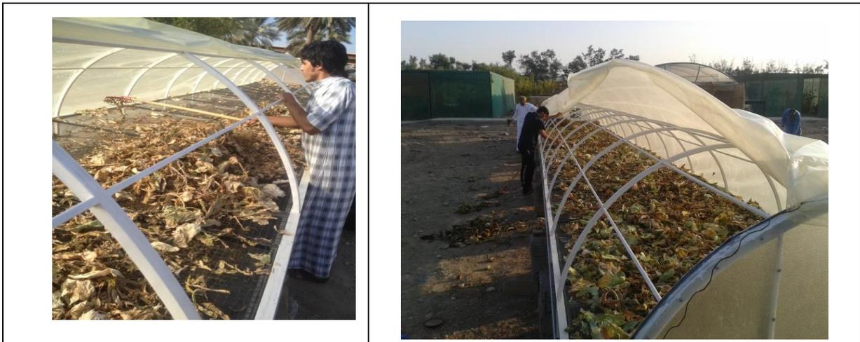
Figure 1. Drying vegetable waste in a drying solar tunnel.
