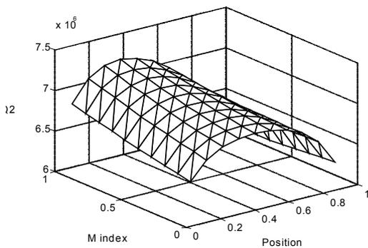
**Figure 8.** Reactive power flow  $Q_2$  for various various Modulation index.
