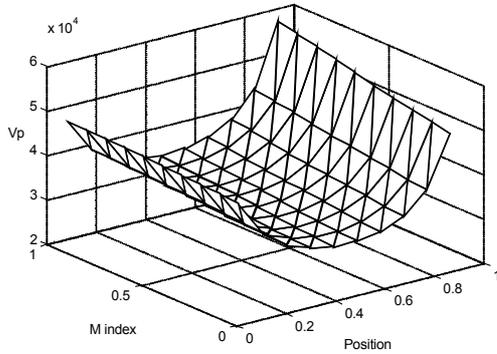
**Figure 4.** Terminal voltage  $V_p$  for various various Modulations index.
