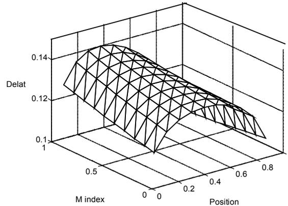
**Figure 10.** Load angle ( $\delta$ ) for various Modulation index.
