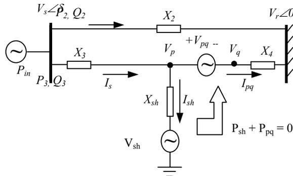
Figure 2. Single Line Diagram of the Study System.
