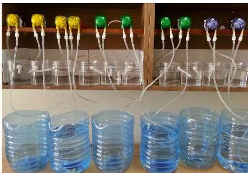
**Figure 1.** Experimental set up showing: peristaltic pumps at the top; mosquito jars in middle row; predator containers alternating with waste jars on bottom row.
