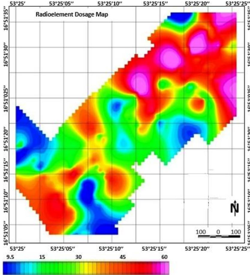
Figure 2. Contour image of radioelement dose (nGy/h) recorded by Gamma ray spectrometer.
