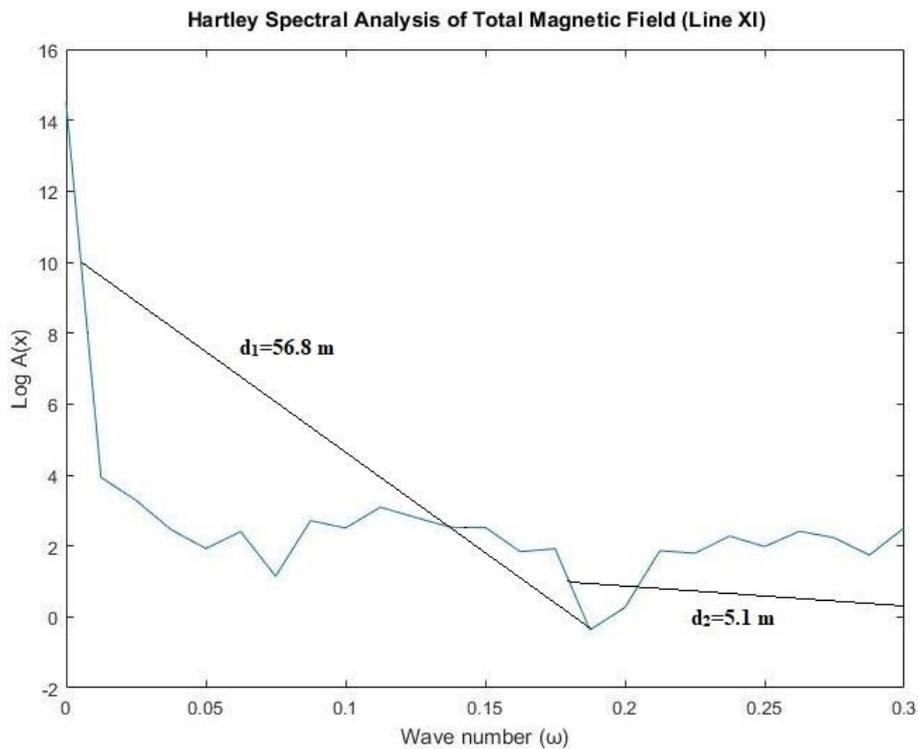
Figure 7. Hartley spectral analysis of total magnetic anomaly of line-VI indicating the depth to subsurface fault.
