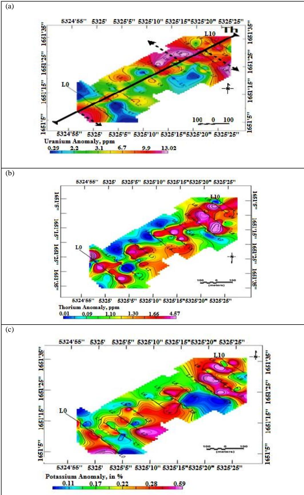
Figure 3. Contour image of concentration in ppm of (a) Uranium (b) Thorium and (c) Potassium recorded by Gamma ray spectrometer.
