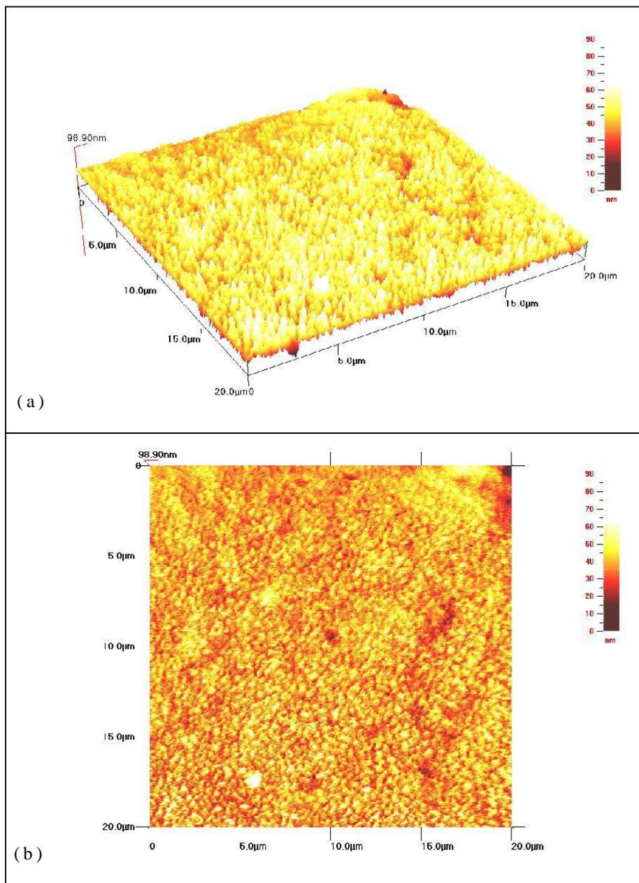
Figure 1. 3-dimesional (Figure 1a) and 2-dimensional (Figure 1b) AFM image of CuS thin films deposited for 30 min.
