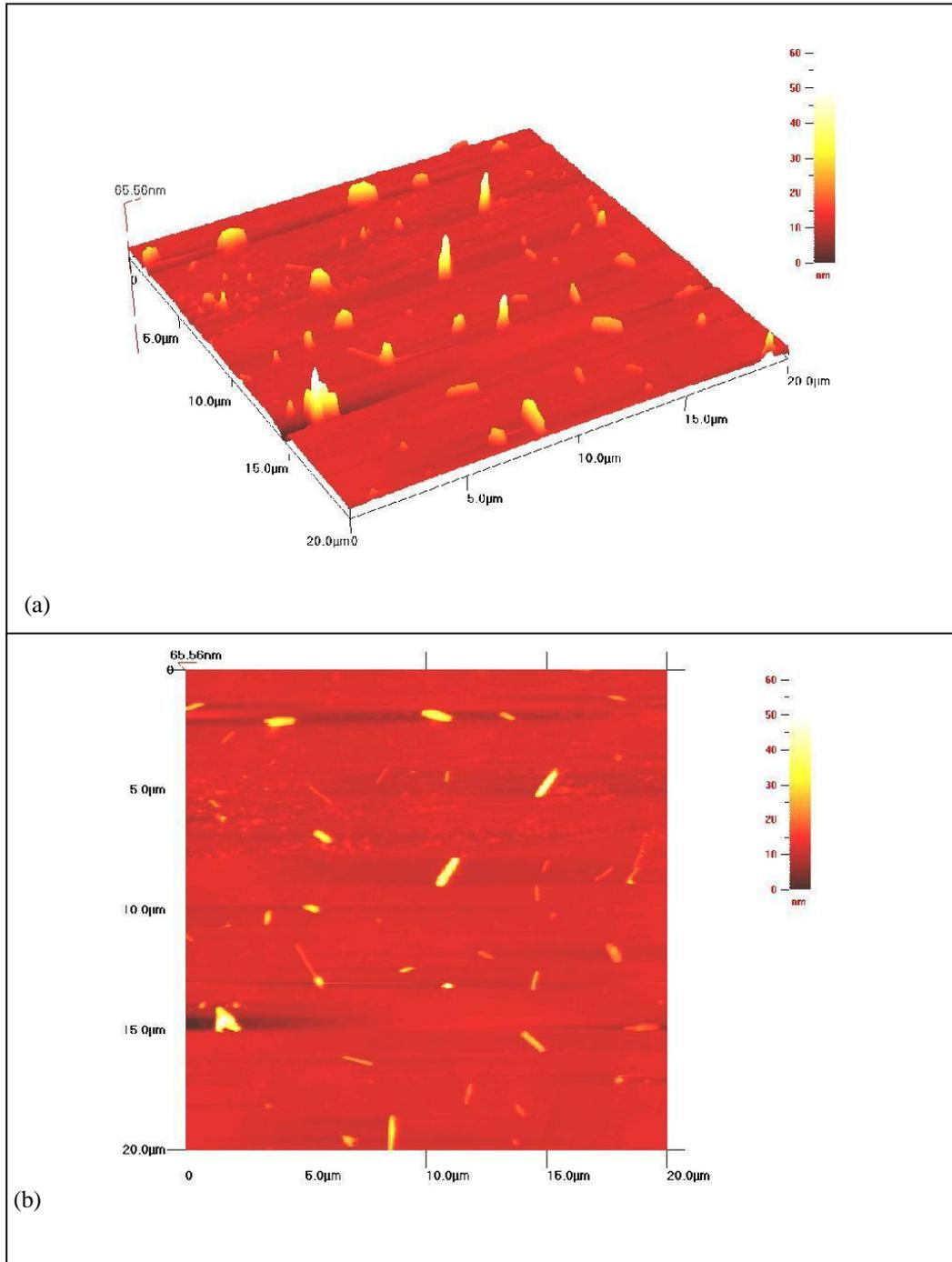
Figure 6. 3-dimensional (Figure 6a) and 2-dimensional (Figure 6b) AFM images of CuS thin films deposited for 180 min.
