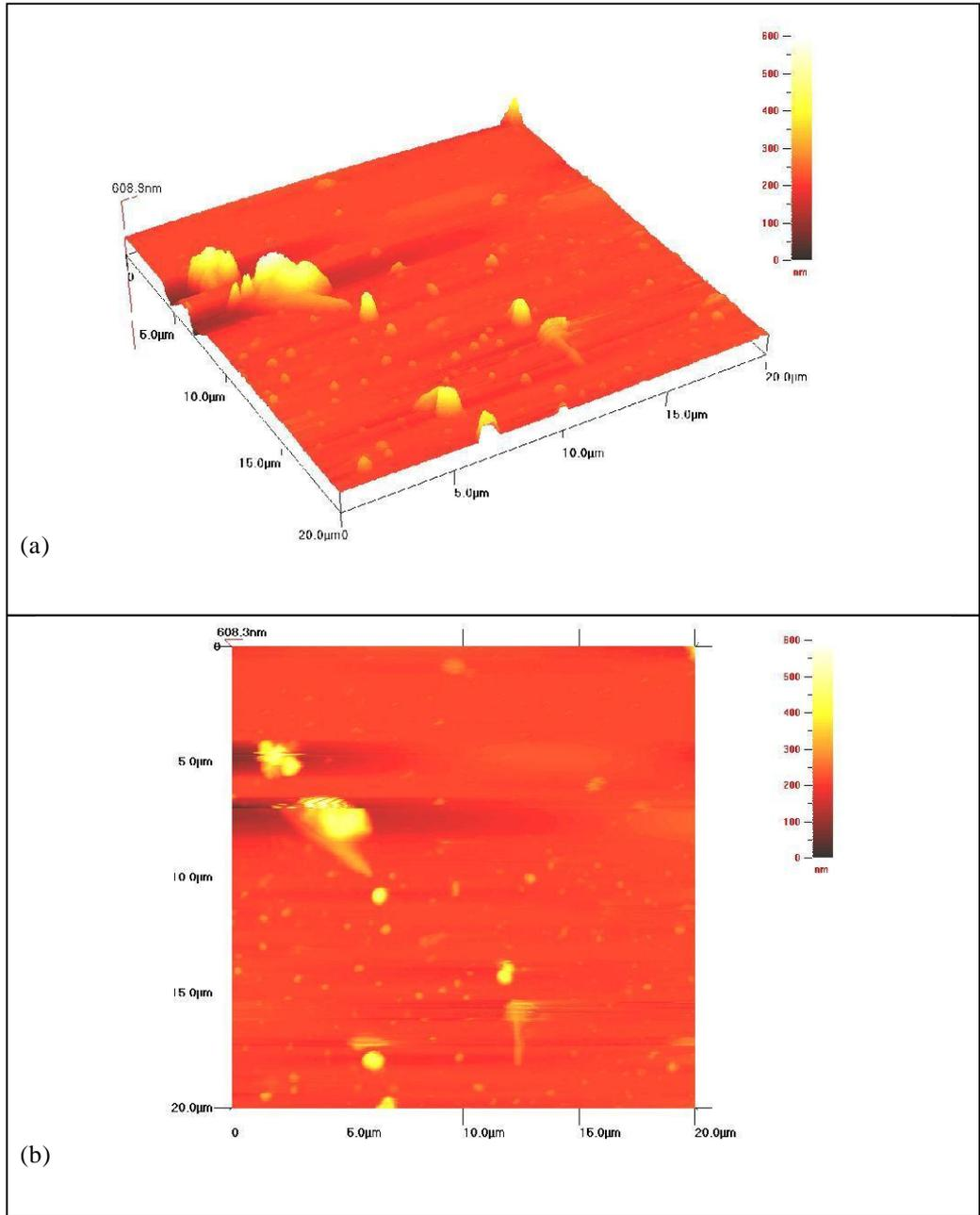
Figure 3. 3-dimensional (Figure 3a) and 2-dimensional (Figure 3b) AFM image of CuS thin films deposited for 90 min.
