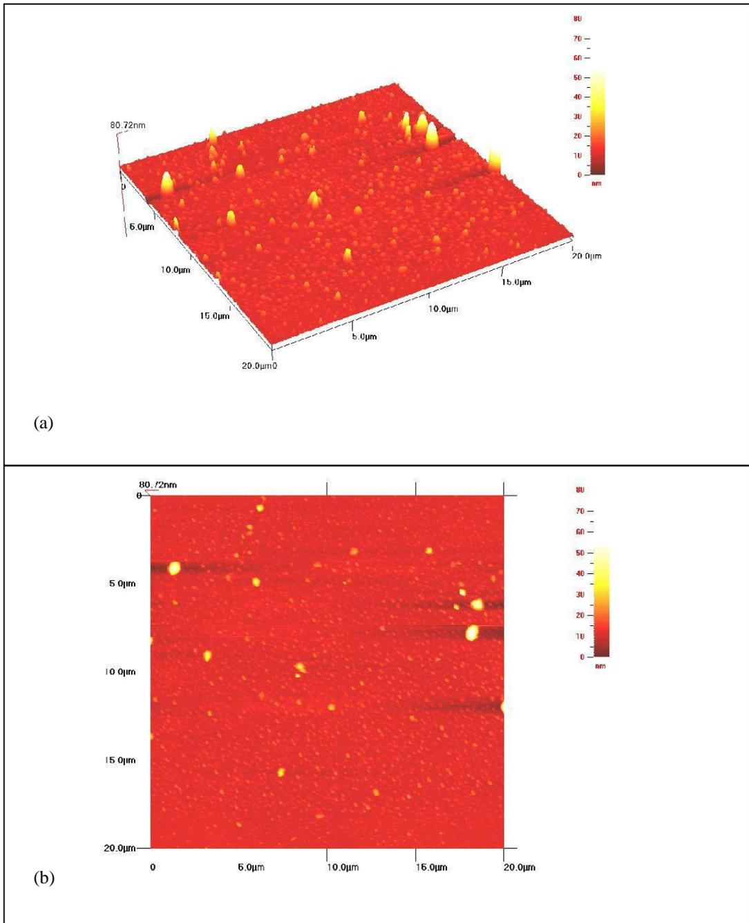
Figure 5. 3-dimensional (Figure 5a) and 2-dimensional (Figure 5b) AFM images of CuS thin films deposited for 150 min.
