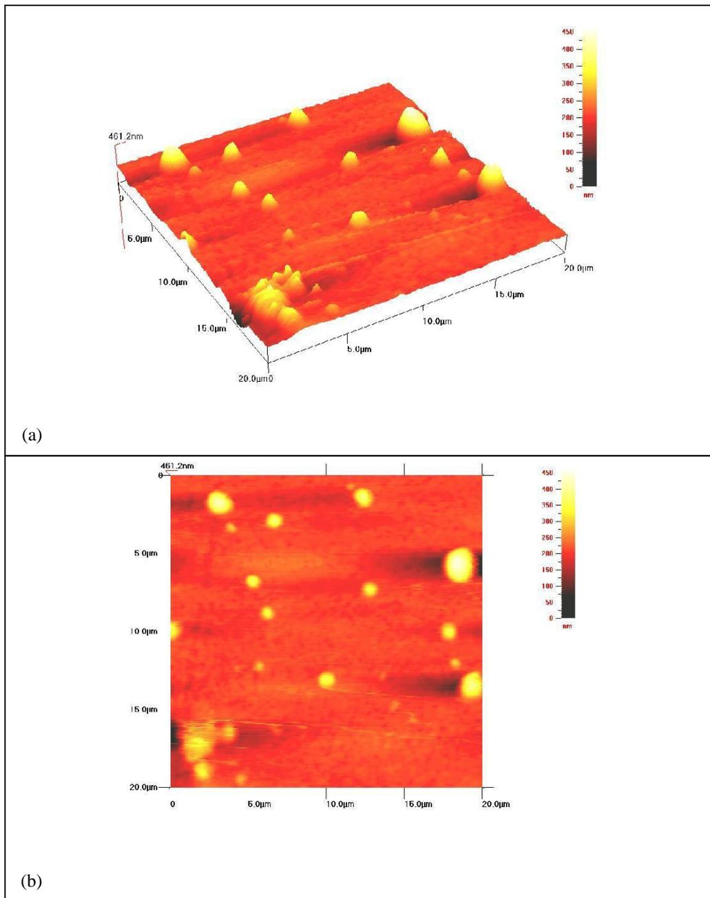
Figure 4. 3-dimensional (Figure 4a) and 2-dimensional (Figure 4b) AFM images of CuS thin films deposited for 120 min.
