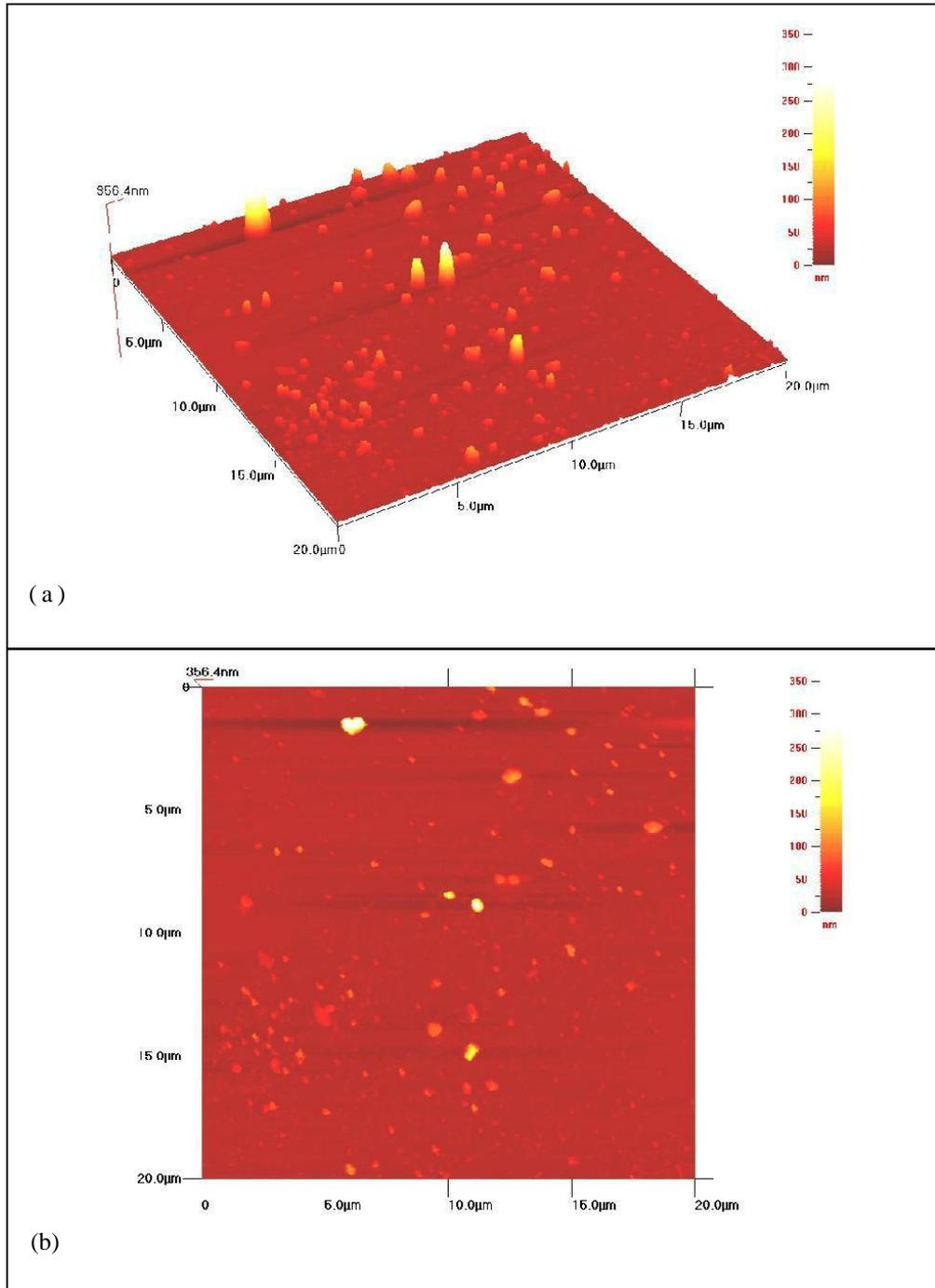
Figure 2. 3-dimensional (Figure 2a) and 2-dimensional (Figure 2b) AFM image of CuS thin films deposited for 60 min.
