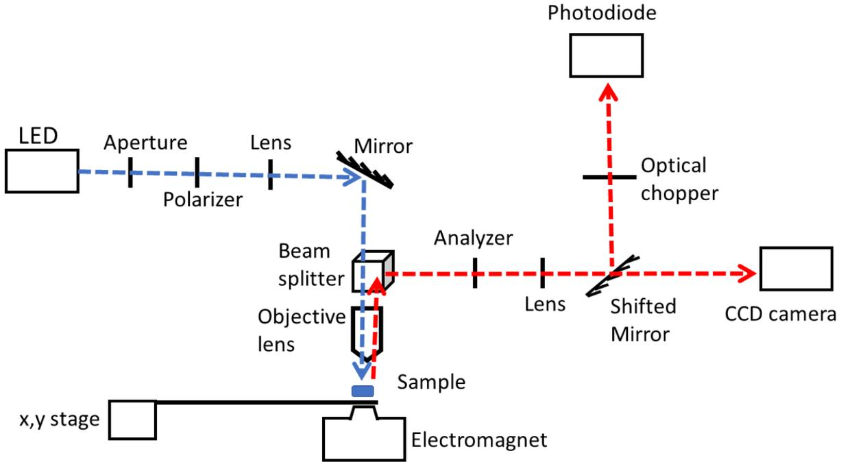
**Figure 1.** A schematic drawing of the MOKE microscope set up.
