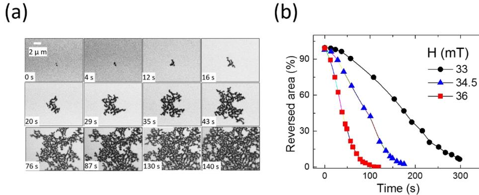
**Figure 3.** Time-dependent magnetization (a) MOKE images of  $10 \mu\text{m} \times 11 \mu\text{m}$  captured after applying a magnetic field of  $33 \text{ mT}$ . (b) Reversed area of the magnetic domains versus time curves plotted after the application of various reverse magnetic fields.
