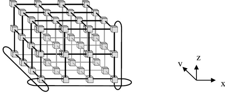
Figure 2. The 3D torus NoC topology.
