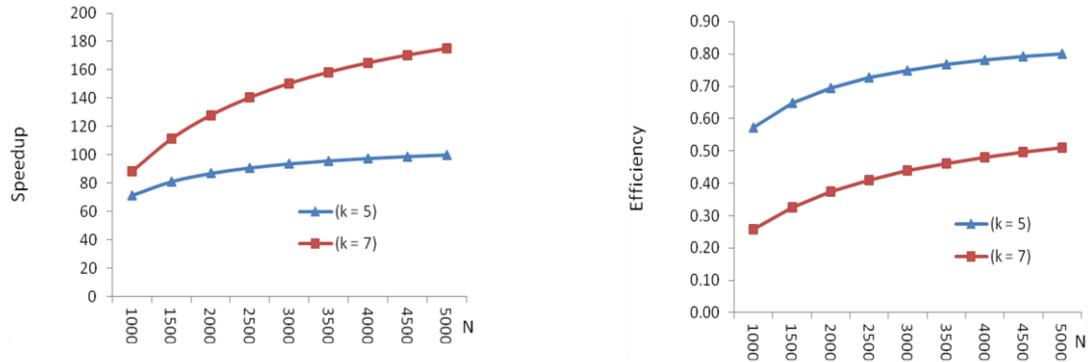
**Figure 8.** Speedup and efficiency of the parallel GS algorithm as a function of  $N$ .
