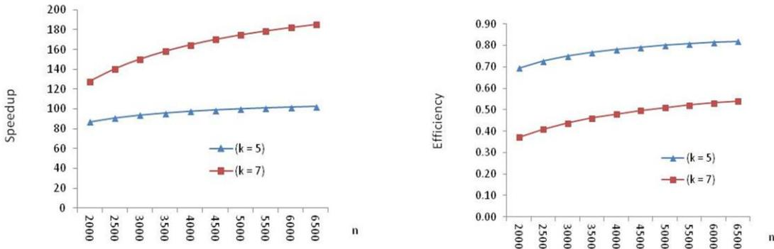
Figure 7. Speedup and efficiency of the parallel GS algorithm as a function of  $n$ .
