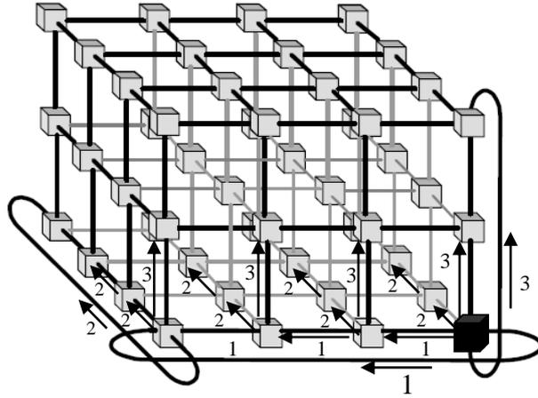
**Figure 5.** Broadcasting on the 3D torus in 3 phases.
