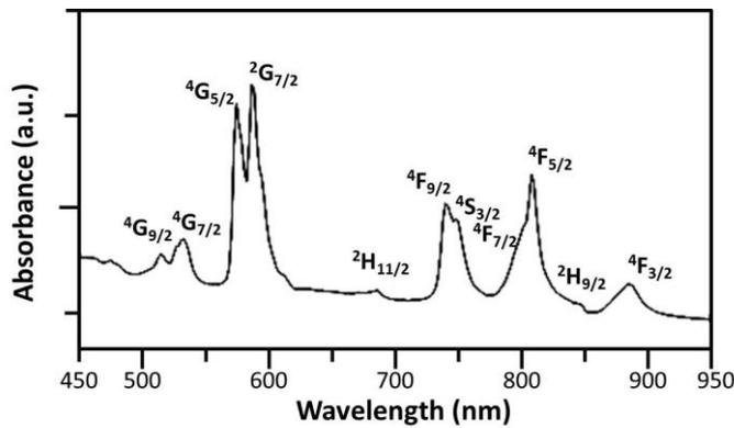
**Figure 1.** Absorption spectra of Nd<sup>3+</sup> in sodium bismuth silicate glass.
