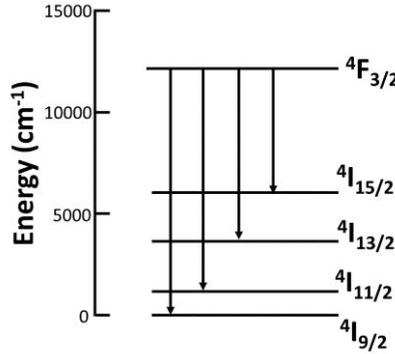
**Figure 2.** Possible radiative channels of  $Nd^{3+}$  from  ${}^4F_{3/2}$  level.
