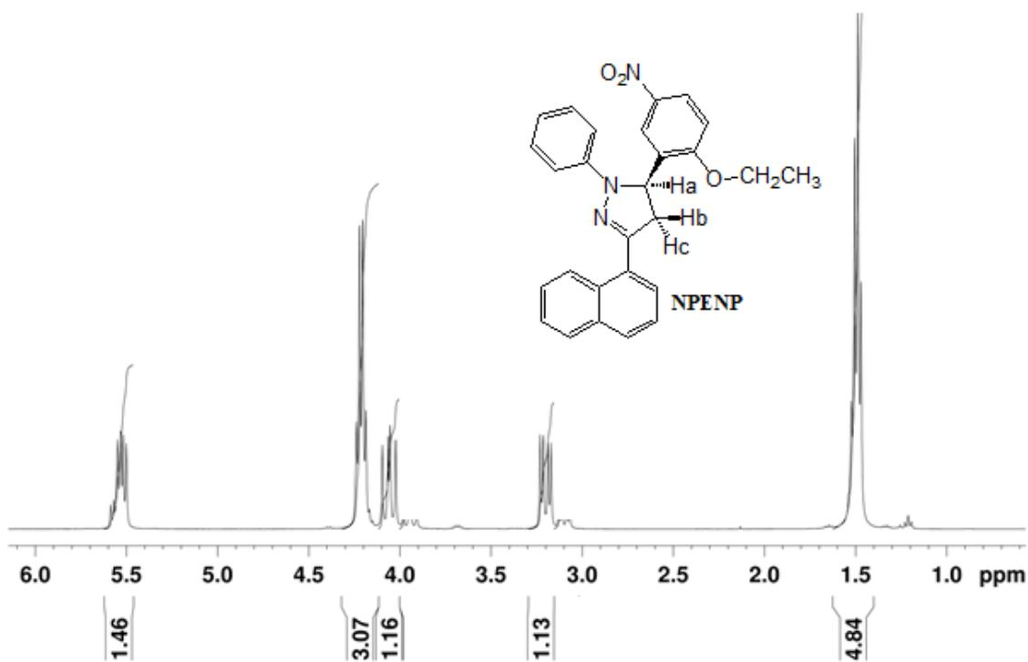
Figure 3. The aliphatic  $^1\text{H}$  NMR spectrum ( $\text{CDCl}_3$ ) of NPENP.
