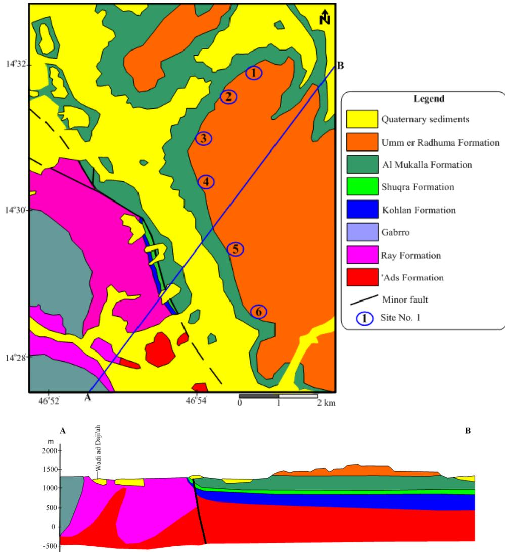
**Figure 3.** Geological map of the study area and cross-section from A-B [14].
