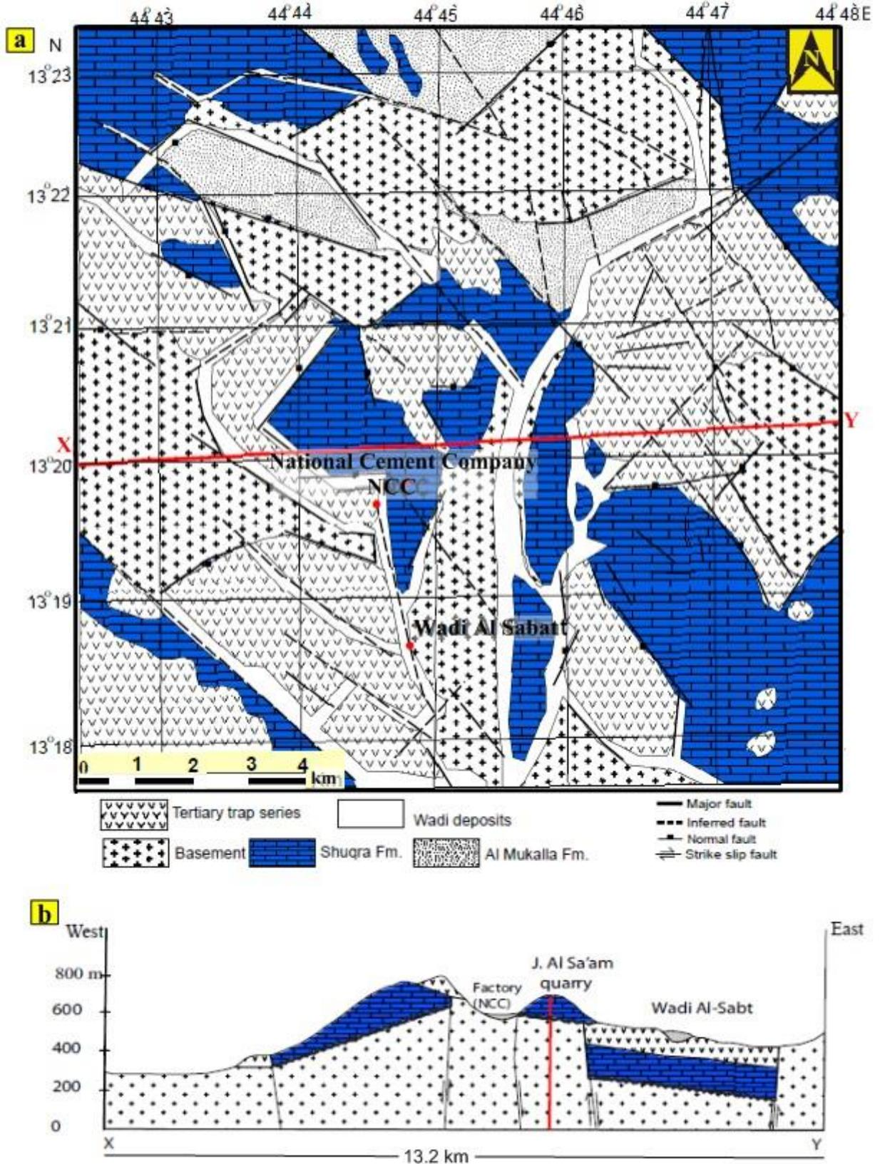
**Figure 8.** a) Detailed geological map of the quarry sites in the Lahj area, and b) Geologic cross-section in the quarry sites.
