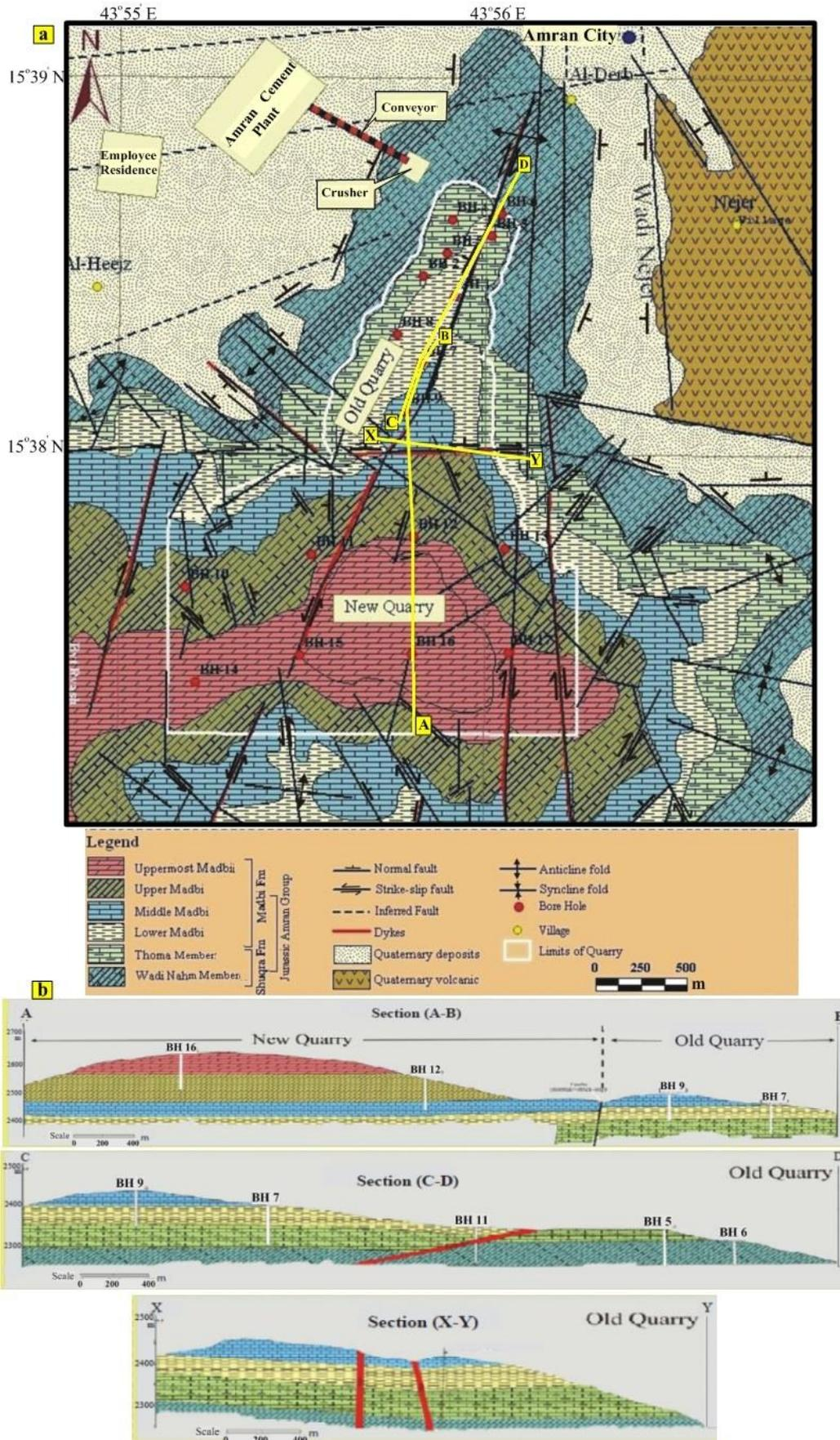
**Figure 2.** a) Detailed geological map of the old and new quarry sites of Amran Cement Plant [19], and b) Geologic cross-sections in the quarry sites [19].
