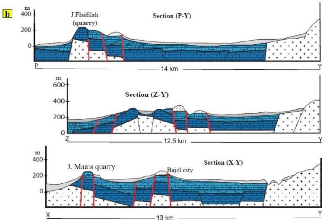
**Figure 4.** a) Detailed geological map of the quarry sites in the Bajel area, and b) Geologic cross-sections in the quarry sites.
