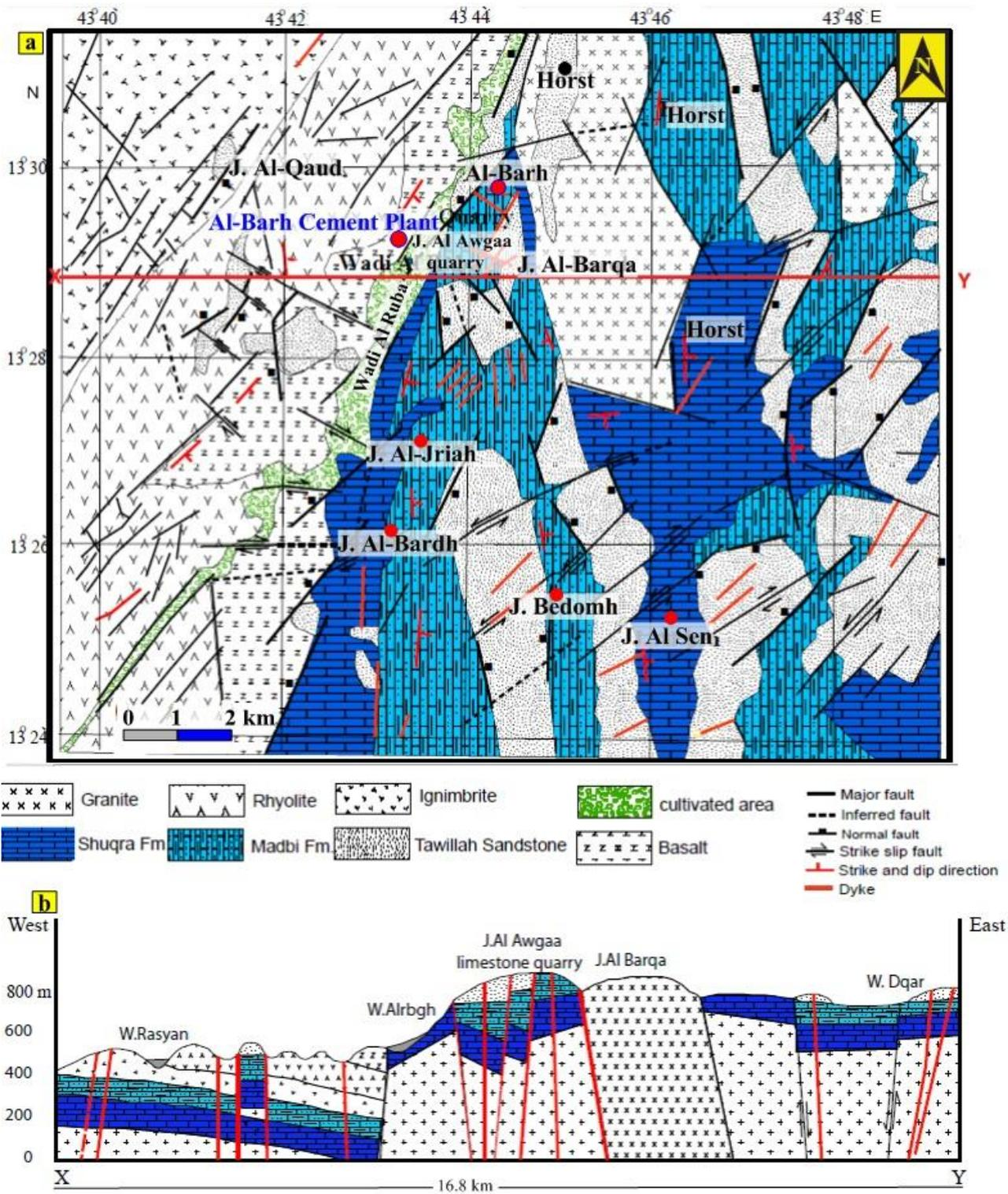
Figure 5. a) Detailed geological map of the quarry sites in the Al-Barh area, and b) Geologic cross-section in the quarry sites.
