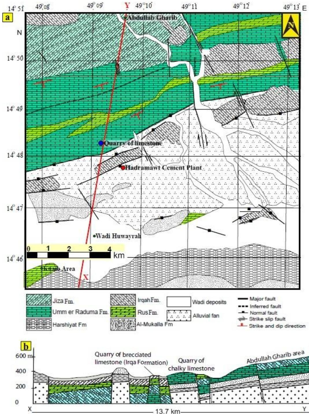
Figure 9. a) Detailed geological map of the quarry sites in the Al-Mukalla area, and b) Geologic cross-section in the quarry sites.
