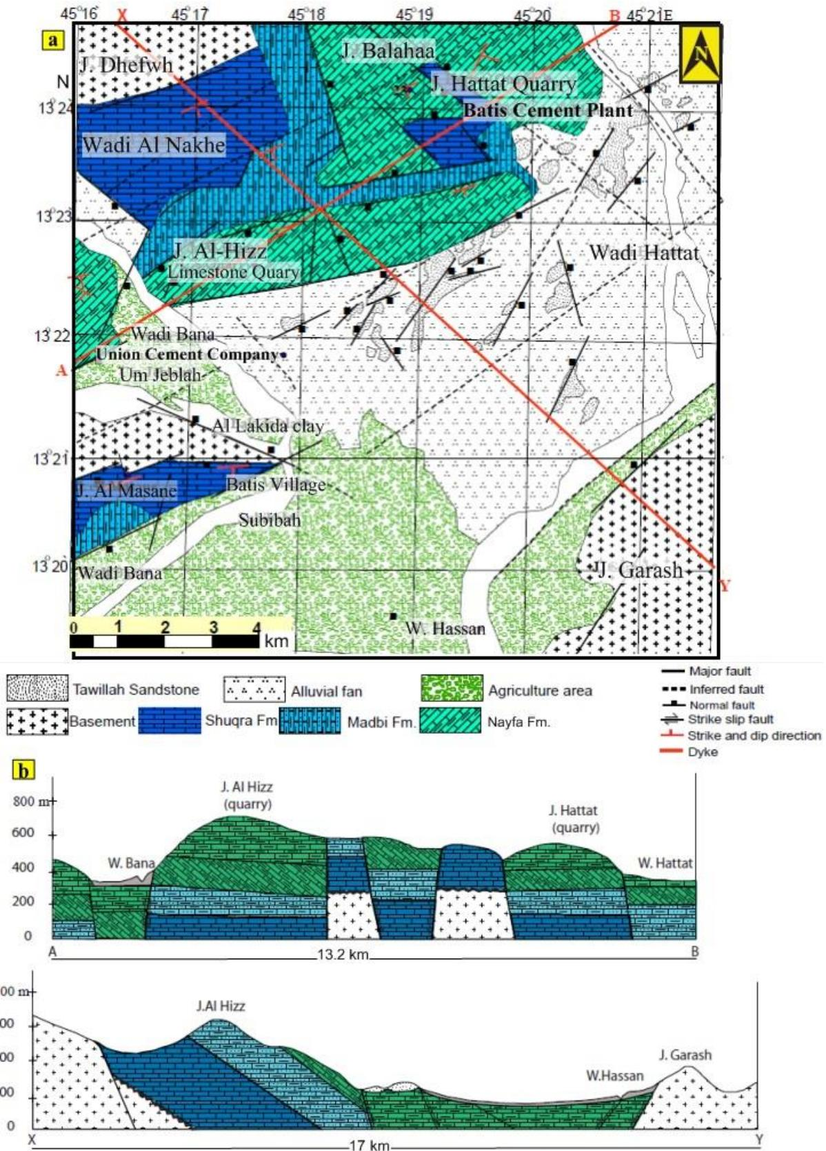
**Figure 7.** a) Detailed geological map of the quarry sites in the Abyan area, and b) Geologic cross-sections of the quarry sites.
