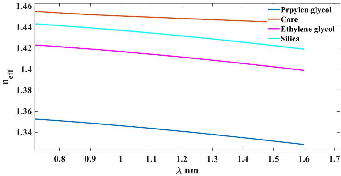
**Figure 2.** The relationship between the refractive indices of  $\text{SiO}_2$ ,  $\text{C}_3\text{H}_8\text{O}_2$  and  $\text{C}_2\text{H}_6\text{O}_2$ .
