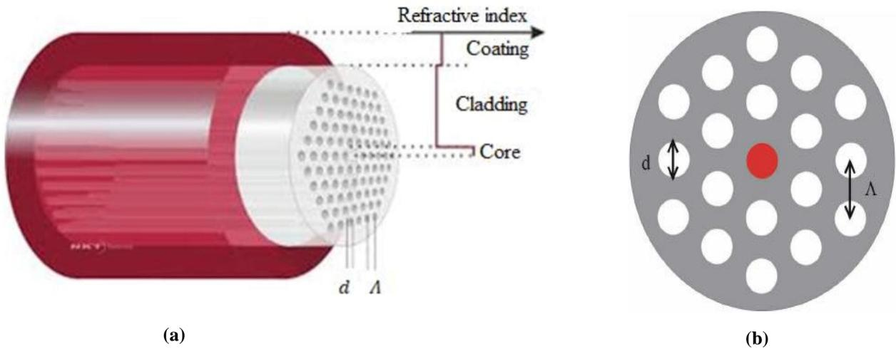
**Figure 1.** (a) Longitudinal section of the photonic crystal fiber, (b) Cross-section of the photonic crystal fiber.
