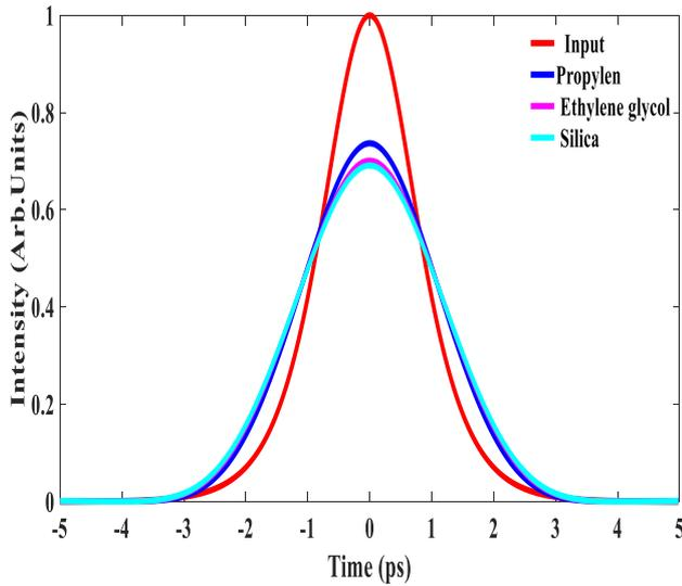
**Figure 4.** The difference in amplitude of different core materials with respect to time.
