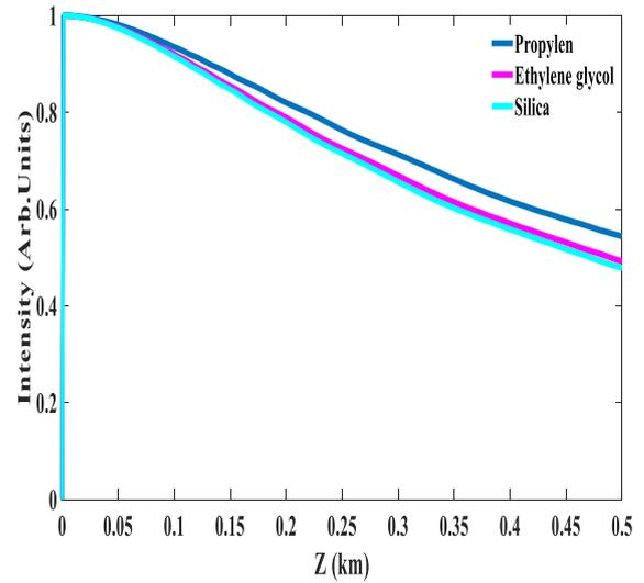
**Figure 5.** The difference in amplitude of different core materials with respect to length.
