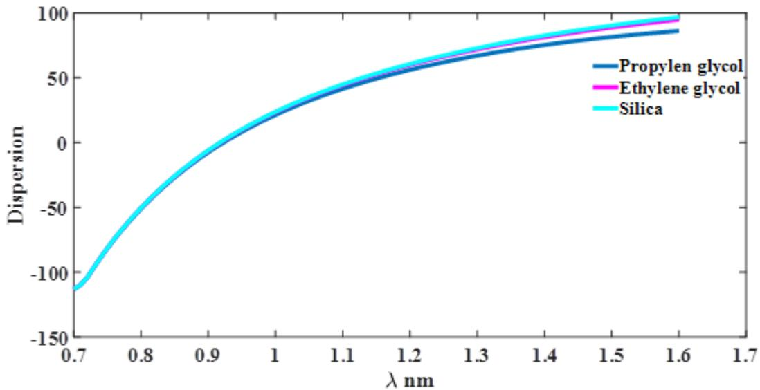
**Figure 3.** The dispersion of cores consisting of  $\text{SiO}_2$ ,  $\text{C}_3\text{H}_8\text{O}_2$ , and  $\text{C}_2\text{H}_6\text{O}_2$ .
