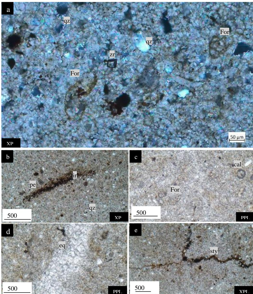
**Figure 12.** Microphotographs of mudstone microfacies show; a- microcrystalline cement, quartz (qz), and undefined foreminifera (For); b- peloids (pe), and burrow filled by iron (ir); c- calcisphere (cal) and foraminifera fragments (For); d- fracture filled by drusy equant calcite (eq), and; e- stylolite (sty).
