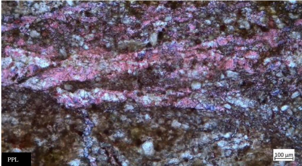
**Figure 8.** Microphotograph of thin section Na3 shows Alizarin Red S and Potassium Ferricyanide stain used for mineral identification. The calcite grains turn to red/pink color. The Fe-rich calcite distinguishes itself from the normal calcite by turning to blue color.
