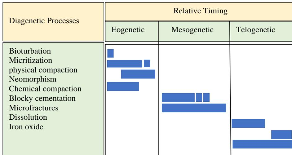
**Figure 13.** The paragenetic sequence of the main diagenetic features detected in the Muti Formation Nakhal section (Na). Note: small squares indicate not knowing the process's end time.
