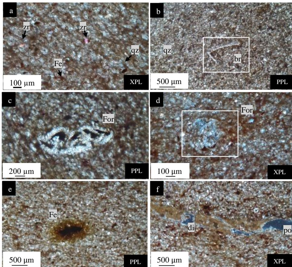
**Figure 11.** Microphotographs of arenaceous wackestone microfacies showing a- micritic mud and with iron oxides at places (Fe) and rare zircon (Zr) and contains detrital quartz (qz), b- brachiopod fragment (br), c&d- planktonic foraminifera, e- iron nodule (Fe), and d- dissolution (di) and porosity (po).
