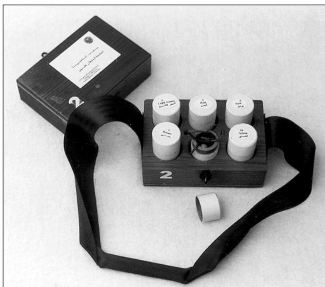
**FIGURE 2.** A wooden box that houses the lead pots containing the capsules.
