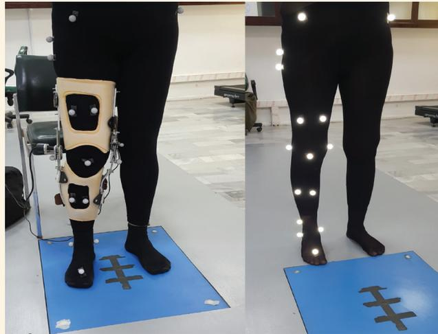
Figure 1: Photographs showing the marker set adopted with the knee orthosis used for three-dimensional gait analysis.
