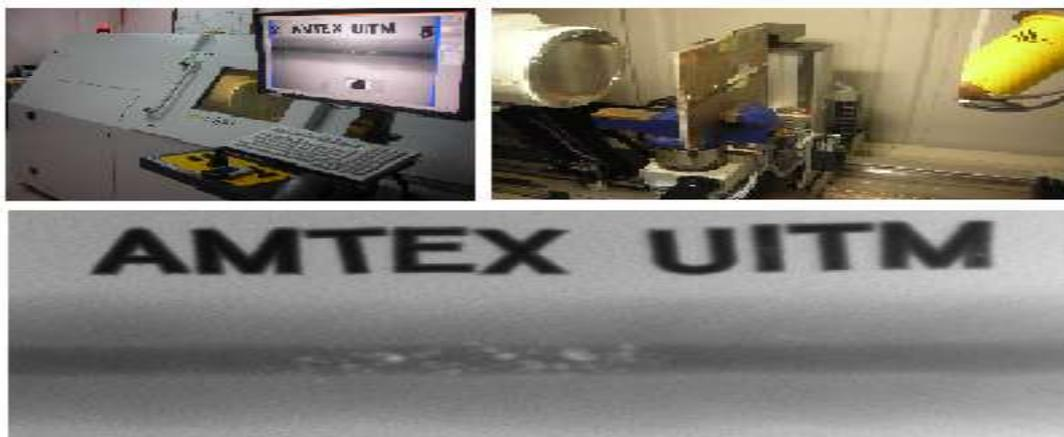
**Figure 2.**  $\mu$ -focussed digital radiograph (top, left), system overview (top, right) and radiographed image using flawed specimen (below) using 180 V, 240 A, FDD = 870 mm and FOD = 270 mm
