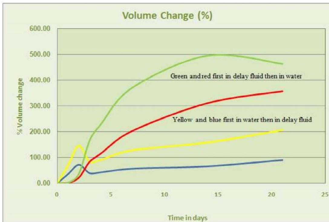
**Figure 4.** Elastomer swelling in water and in swell-delaying fluid
