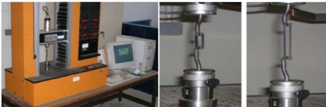
**Figure 1.** Tensile test set-up with specimens at different stages of testing
