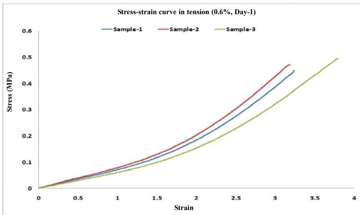
**Figure 9.** Three-sample stress-strain curve under tension at 0.6% salinity after one day of swelling
