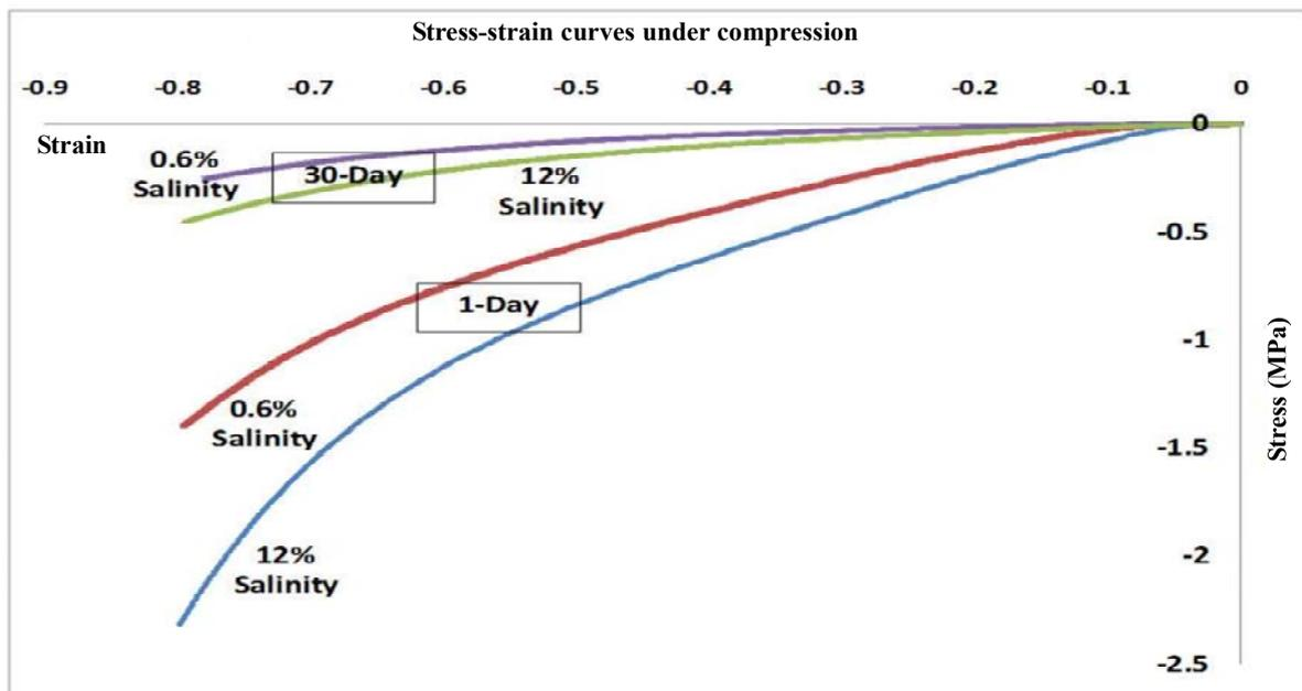
**Figure 16.** Stress-strain curves under compression for two salinities after one and 30 days of swelling
