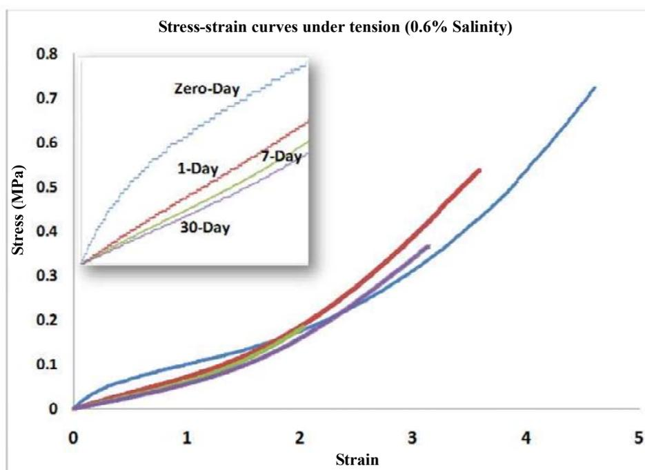
Figure 14. Stress-strain behavior under tension at 0.6% salinity after various swelling periods (Zero, One, 7, and 30 days)
