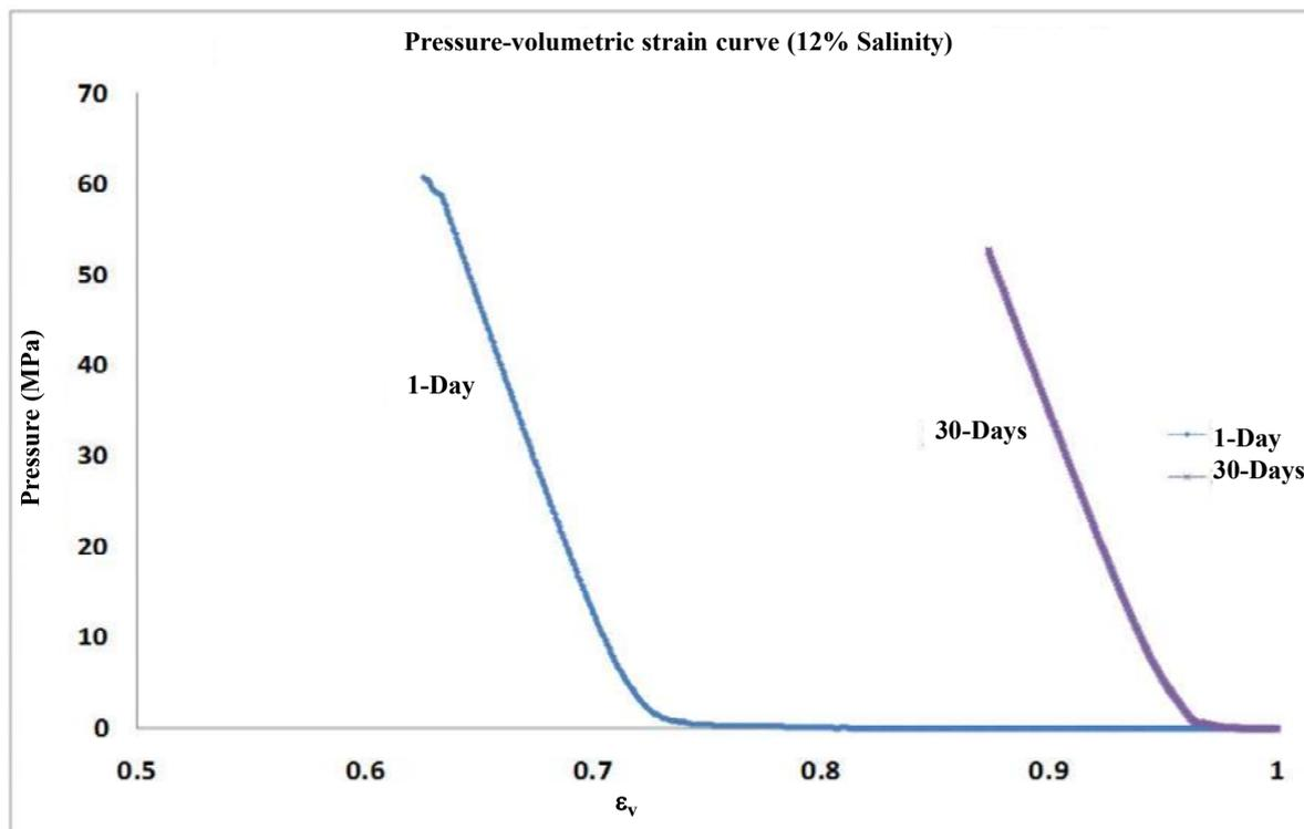
Figure 17. Pressure-volumetric strain curves after one and 30 days of swelling at 12% salinity
