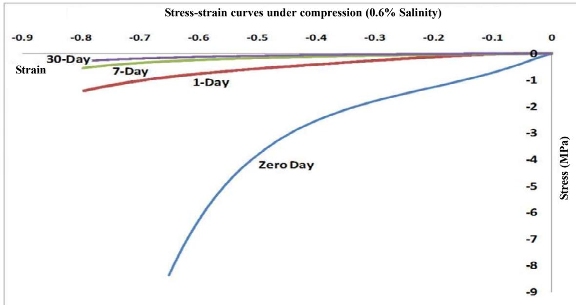
**Figure 15.** Stress-strain behavior under compression at 0.6% salinity after various swelling periods (zero, one, 7 and 30 days)
