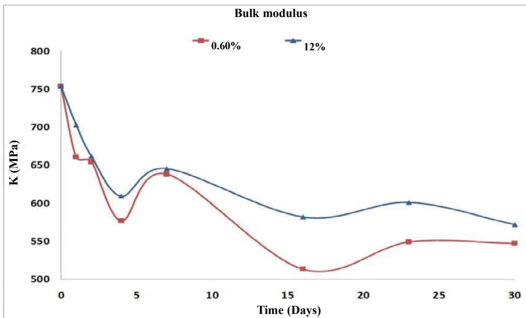
Figure 20. Bulk modulus for both salinities for the full 30-day test period
