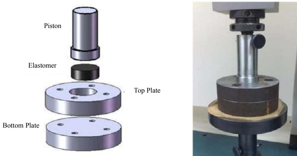
**Figure 3.** Test rig for bulk experiments, designed and fabricated in-house
