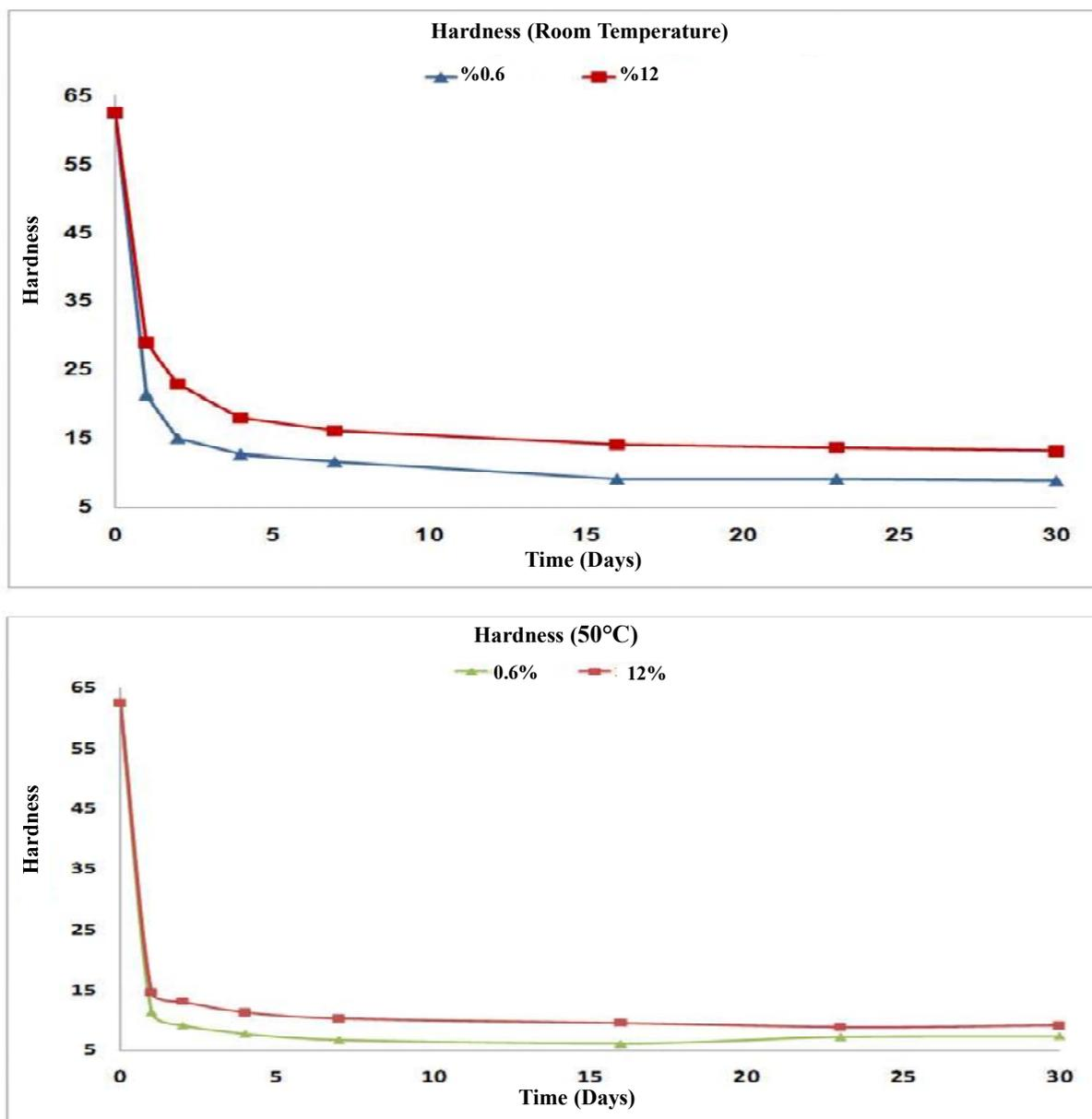
**Figure 7.** Change in hardness over a one-month swelling period at 0.6% and 12% salinity with solution held both at room temperature and 50°C
