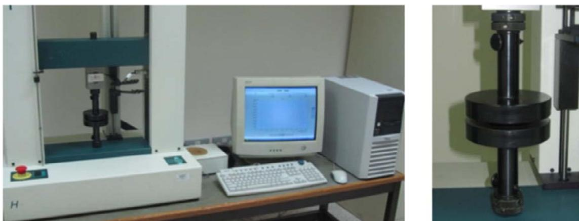
**Figure 2.** Compression test set-up
