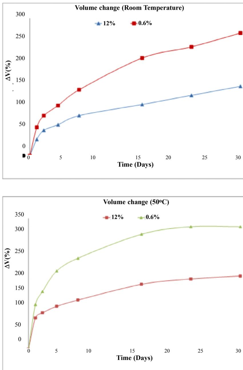
**Figure 5.** Changes in volume after one month of swelling at 0.6% and 12% salinity, held both at room temperature and 50°C
