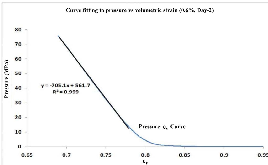
Figure 13. Linear fit to pressure-volumetric strain curve at 0.6% salinity after 2 days of swelling
