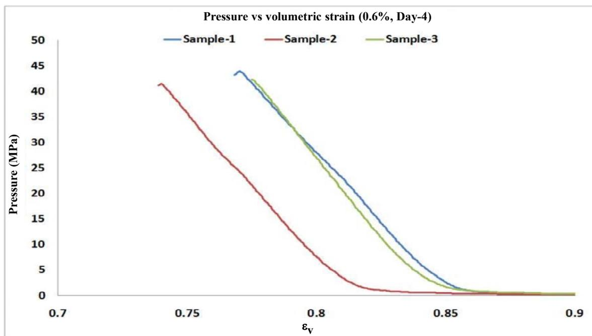
Figure 12. Three-sample pressure-volumetric strain curve at 0.6% salinity after 4 days of swelling
