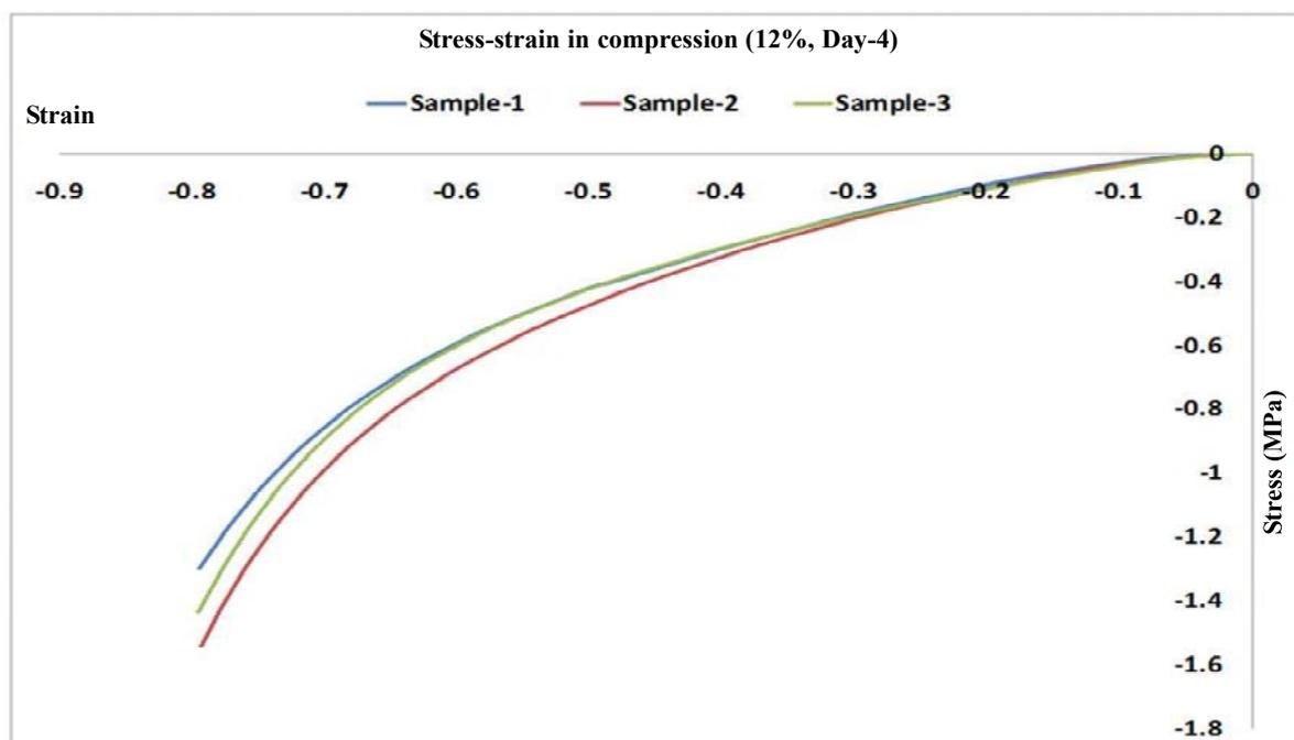
**Figure 10.** Three-sample stress-strain curve under compression at 12% salinity after 4 days of swelling
