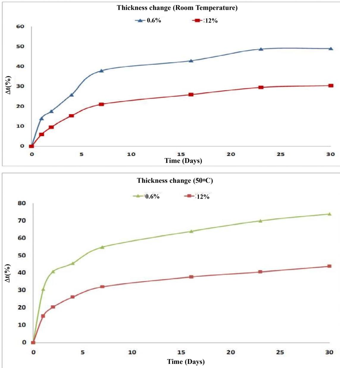
**Figure 6.** Thickness variation for a one-month swelling period with the solution held at 0.6% and 12% salinity at both room temperature and 50°C
