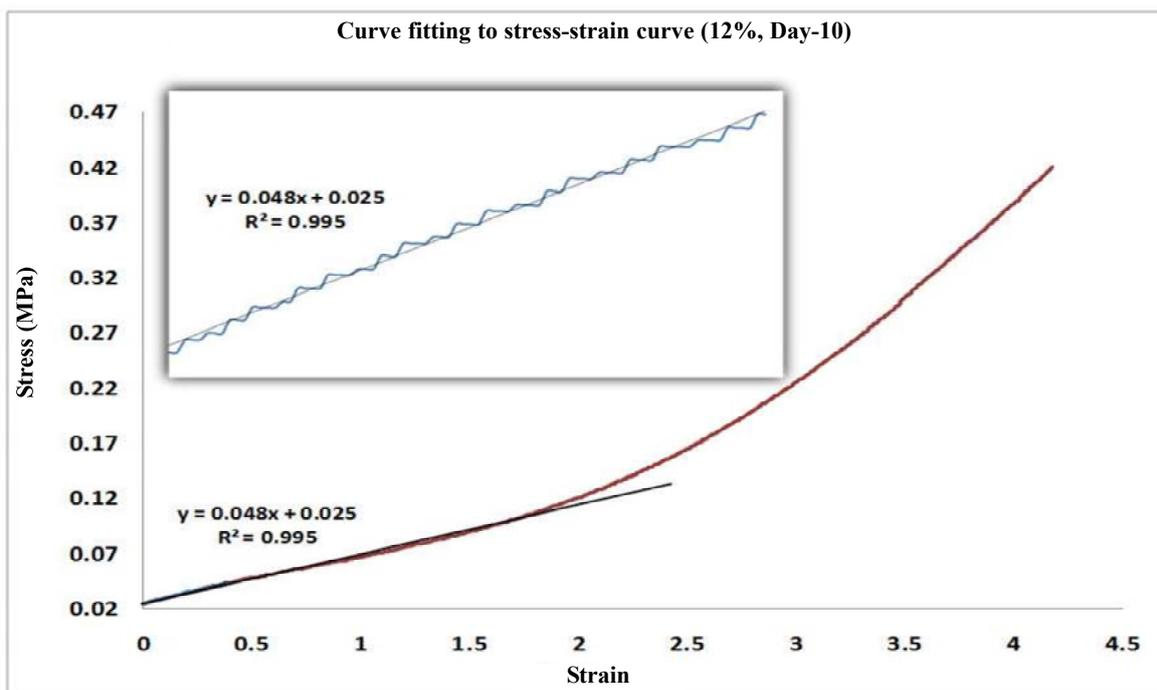
Figure 11. Linear fit to stress-strain curve under tension at 12% salinity after 10 days of swelling
