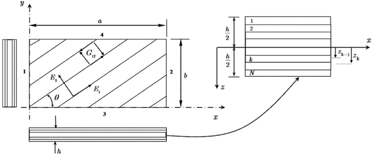
Figure 1. General description of the composite plate model
