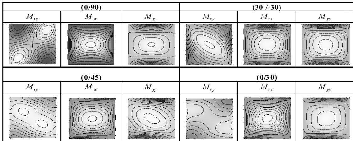
**Figure 2.** Contour plot of moment resultants for different laminated plates with  $S_1S_1C_3C_3$  boundary conditions
