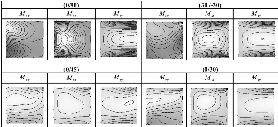
Figure 3. Contour plot of moment resultants for different laminated plates with  $S_1F_4C_3C_3$  boundary conditions
