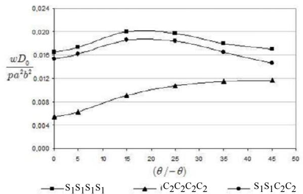
Figure 6. Variation of non-dimensional deflection with fiber orientation angle ( $b/h = 20$ )
