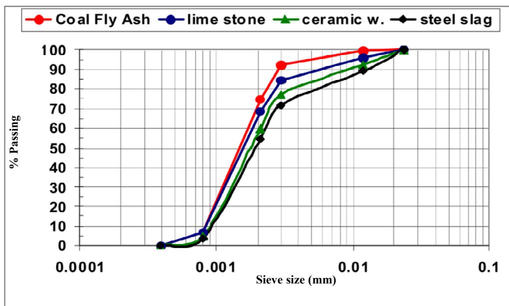
**Figure 4.** Mineral fillers particle size distribution
