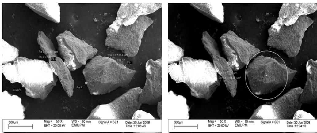
Figure 8. Grain size and particle shape of steel slag at 50 x magnification
