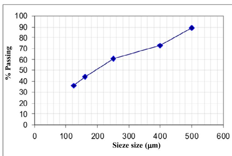
Figure 2. Particle size distribution of cellulose oil palm fiber
