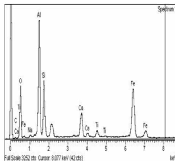
**Figure 12.** Chemical composition of steel slag
