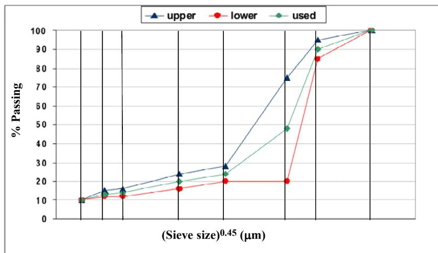
Figure 1. Aggregate particle size distribution
