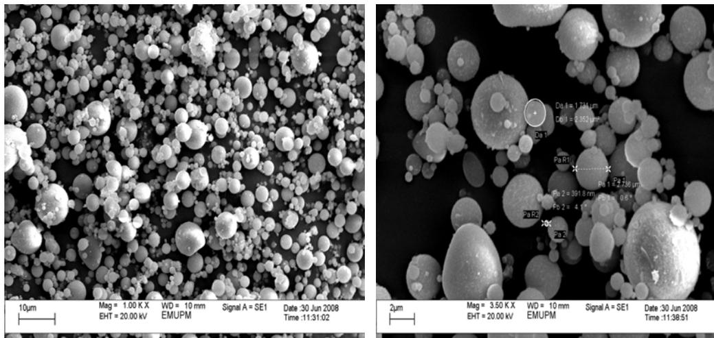
**Figure 5.** Fly ash particles at 1,000 x and at 3,500 x magnification
