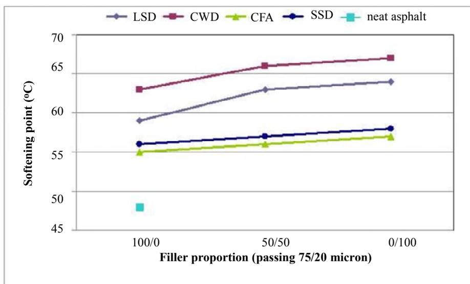
Figure 17. Softening point of neat asphalt and mastics
