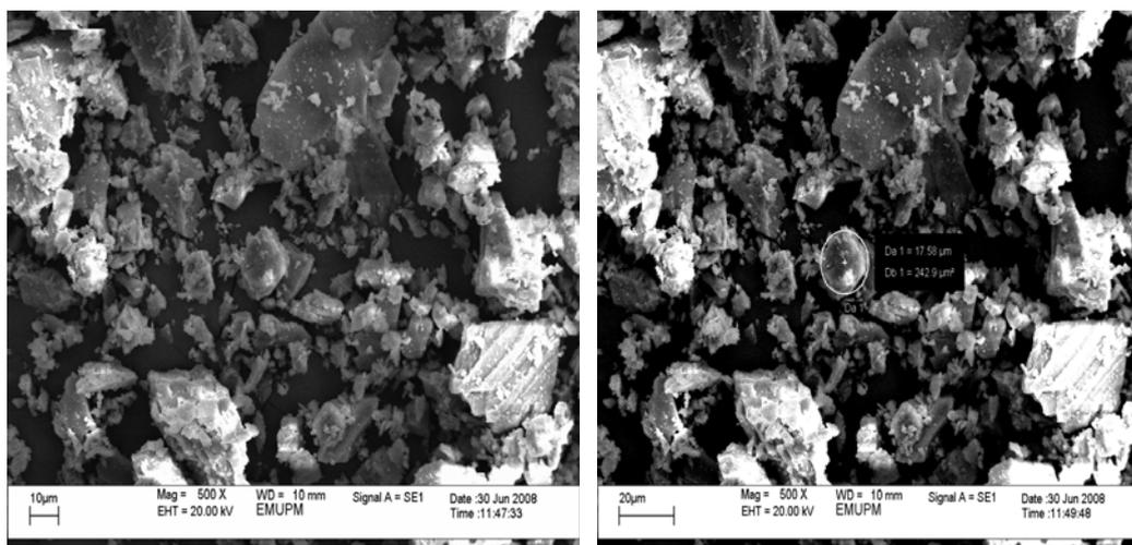
**Figure 6.** Grain size and particle shape of limestone dust at 500 x magnification
