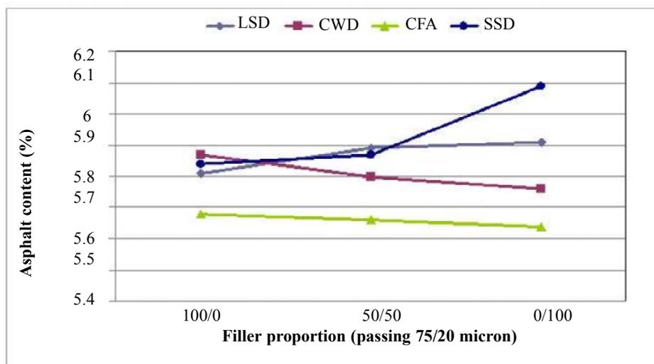
Figure 19. Asphalt content vs filler type
