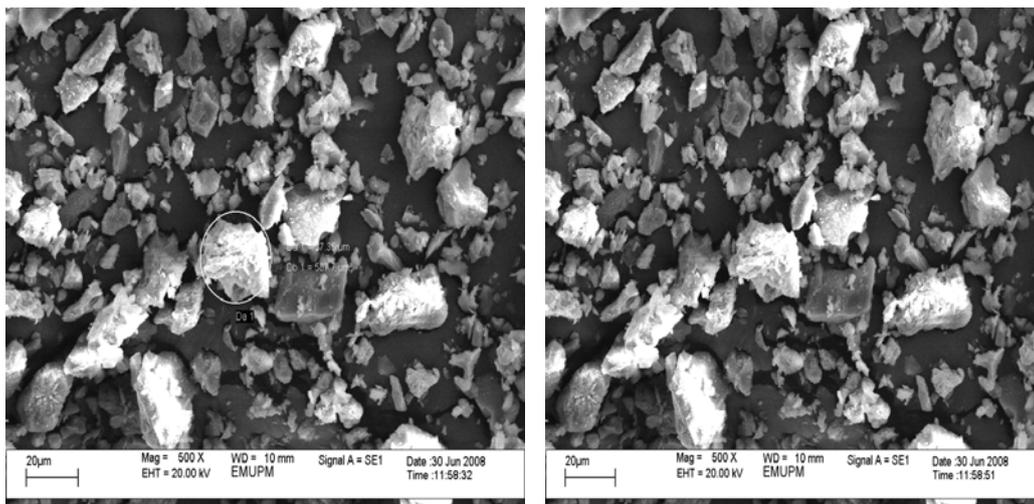
Figure 7. Grain size and particle shape of ceramic waste dust at 500 x magnification
