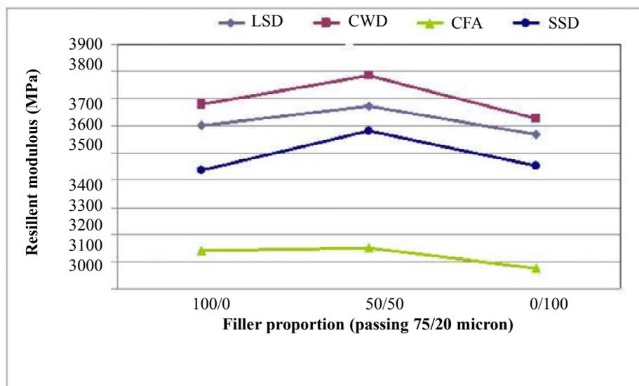
Figure 23. Resilient modulus vs filler type and combination
