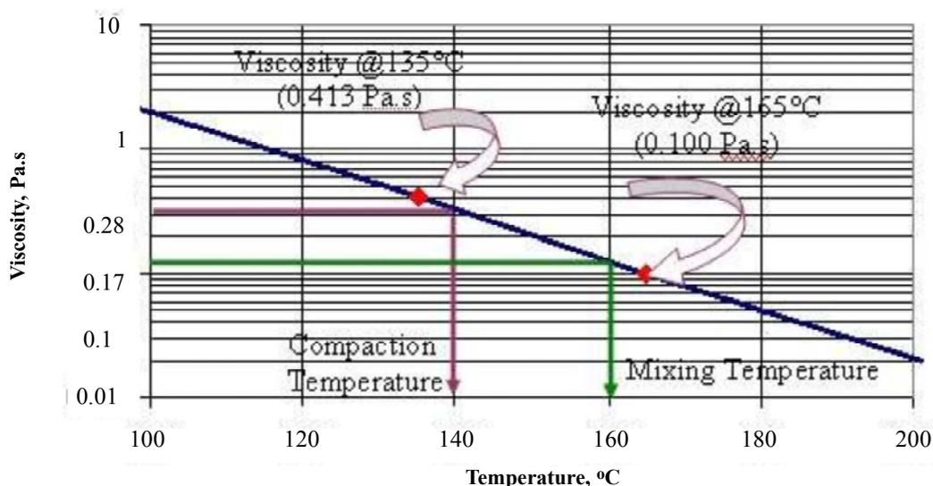
Figure 18. Viscosity - temperature relationships for asphalt binder
