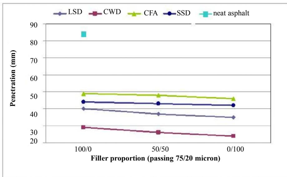
Figure 16. Penetration of neat asphalt and mastics
