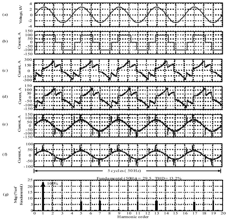
Figure 8. Configuration #3 at  $\alpha=45^\circ$ ; (a) supply phase voltage,  $v_s$ , (b) converter current,  $i_p$ , (c) filter current,  $i_f$ , (d) compensation current,  $i_c$ , (e) compensated secondary current,  $i_{sec}$ , (f) compensated supply current,  $i_s$ , (g) spectrum of compensated supply current.
