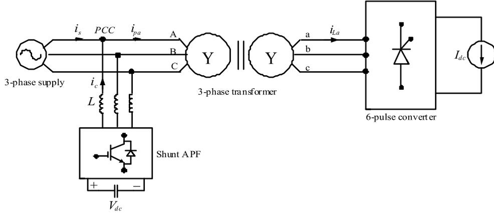
**Figure 1.** Configuration # 1 APF connected to the primary side.
