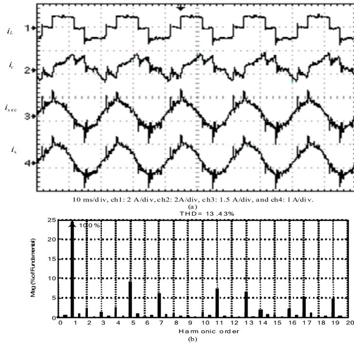
**Figure 6.** Configuration #2 practical results at  $\alpha = 45^\circ$ : (a) current waveforms and (b) spectrum of compensated supply current  $i_s$ .
