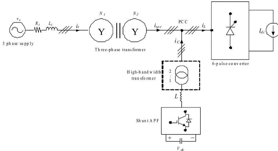
Figure 7. Configuration #3 APF in the secondary side with a high quality stepdown transformer.
