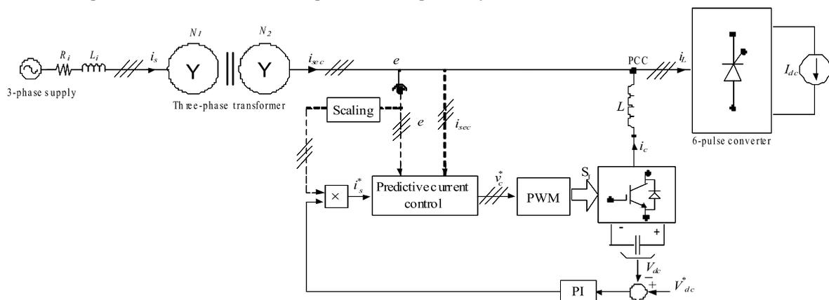
**Figure 4.** Configuration #2 APF on the secondary side.
