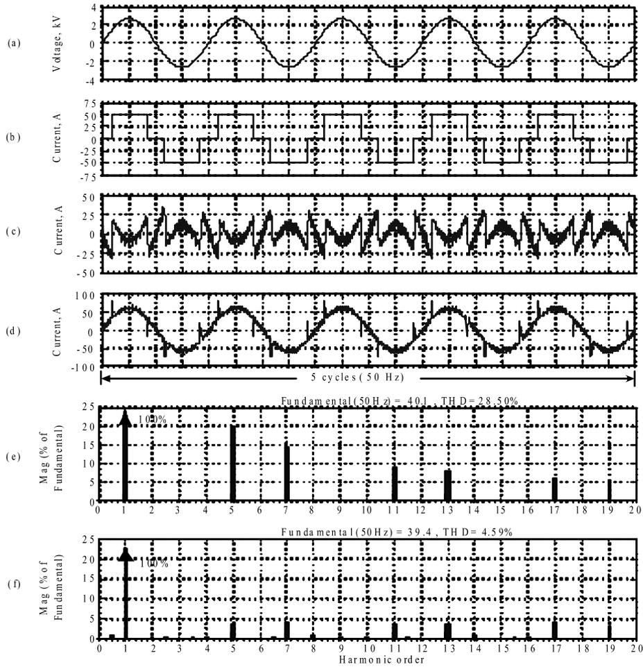
**Figure 2.** Configuration #1 at  $\alpha = 0^\circ$ : (a) supply phase voltage,  $v_s$ , (b) transformer primary current,  $i_p$ , (c) filter current,  $i_c$ , (d) compensated supply current,  $i_s$ , (e) spectrum of converter current, and (f) spectrum of compensated supply current.
