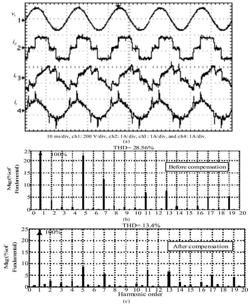
**Figure 3.** Configuration #1 practical results at  $\alpha = 45^\circ$ : (a) current waveforms, and (b) & (c) supply current spectrum before and after compensation, respectively.
