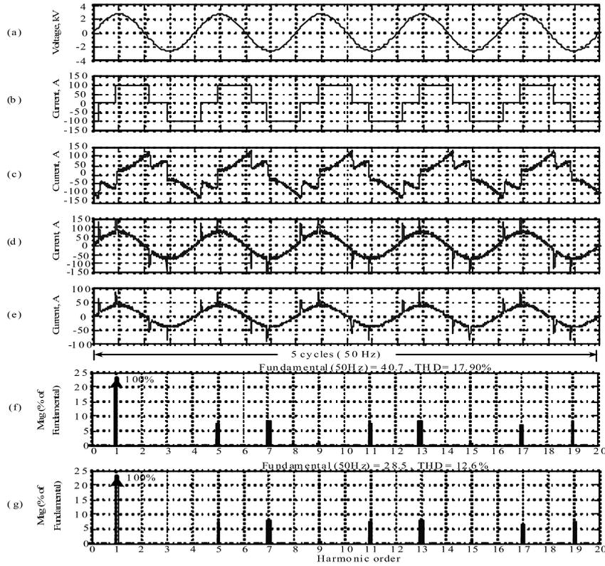
**Figure 5.** Configuration #2 for  $\alpha = 45^\circ$ : (a) supply phase voltage,  $v_s$ , (b) converter current,  $i_b$ , (c) filter current  $i_s$ , (d) compensated secondary current,  $i_{sec}$ , (e) compensated supply current,  $i_{sec}$ , (f) spectrum of  $i_{sec}$ , (g) spectrum of  $i_s$ .
