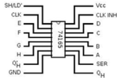
**Figure 2.** A Logisim representation of the in-house built parallel load serial out shift register IC 74165.
