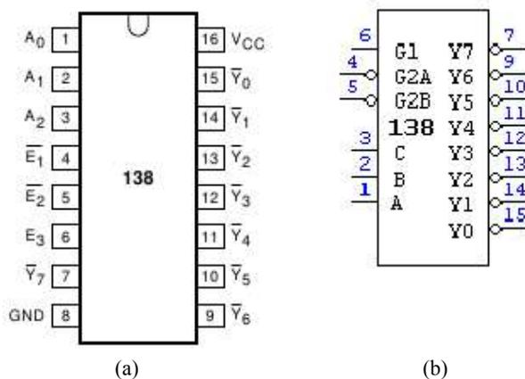
**Figure 1.** The difference between the actual chip layout (a) and LogicWorks layout (b).
