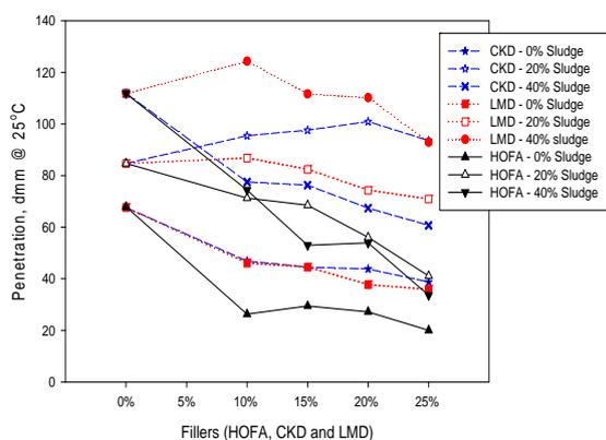
Figure 7. Penetration of the Oil-Sludge Asphalt Mastics.
