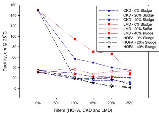
Figure 6. Ductility of the Oil-Sludge Asphalt.
