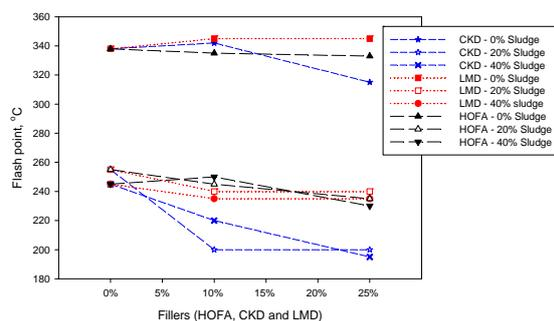
Figure 8. Flash Point of the Oil-Sludge Asphalt Mastics.
