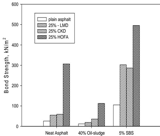
Figure 10. Bond Strength of Fillers, Oil-Sludge And SBS Asphalt Mastics.
