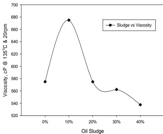
**Figure 3.** Viscosity Vs. Oil-Sludge.
