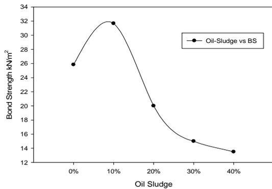
Figure 9. Bond Strength Vs. Oil-Sludge.
