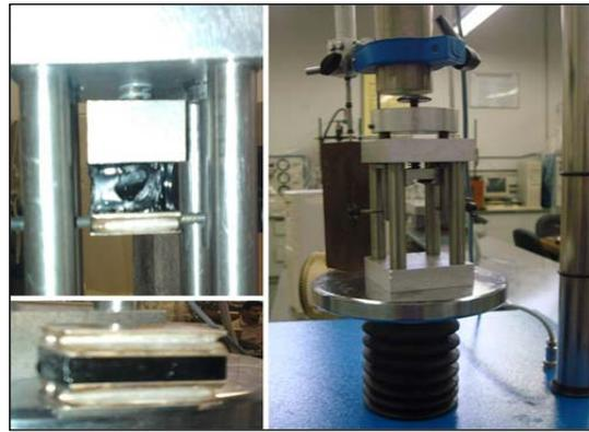
**Figure 1.** Bond Strength Test Setup.
