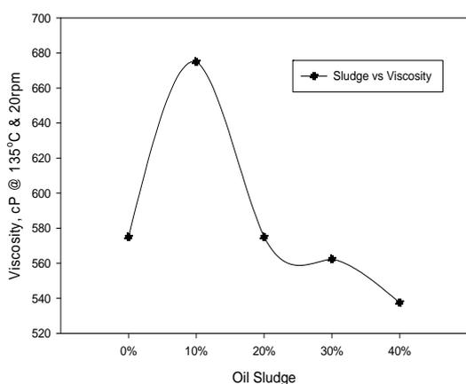
**Figure 3.** Viscosity Vs. Oil-Sludge.
