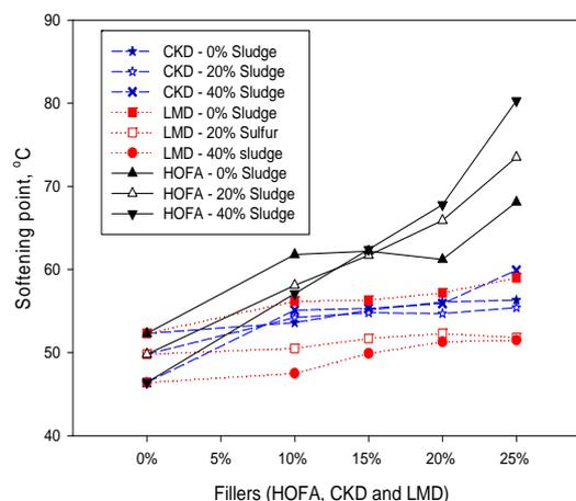
**Figure 4.** Softening Point of the Oil-Sludge Asphalt Mastics.
