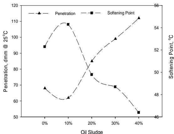
**Figure 2.** Penetration and Softening Point Vs. Oil-Sludge.
