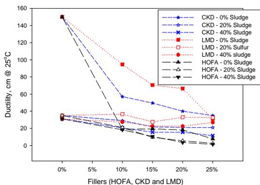
Figure 6. Ductility of the Oil-Sludge Asphalt.
