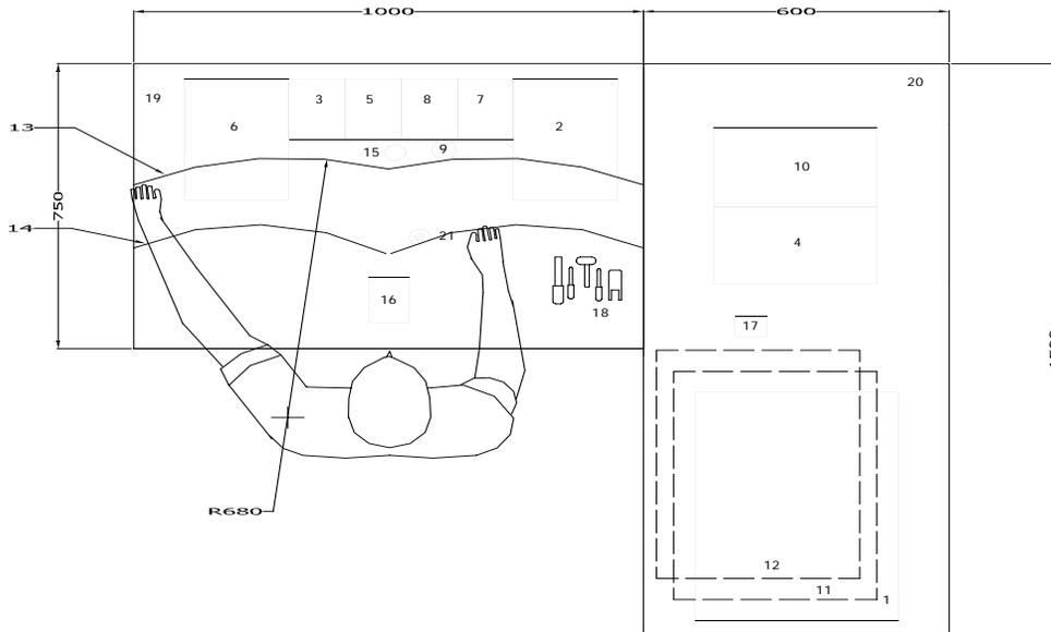
Legend: 1. Incoming bin (600x400); 2. Terminal lever bin (320x205); 3. Terminal clamp bin (140x110); 4. 3-pole body bin; 5. Handle base bin; 6. Handle springs, long screws, cover parts bin; 7. Handles bin; 8. Tripping lever bin; 9. Tripping lever springs bin; 10. Chutes; 11. Covers bin; 12. Outgoing bin; 13. Maximum reach; 14. Normal reach; 15. Grease container; 16. Assembly area; 17. Fixture; 18. Tool area; 19. Assembly table; 20. Side table; 21. Power screwdriver.
