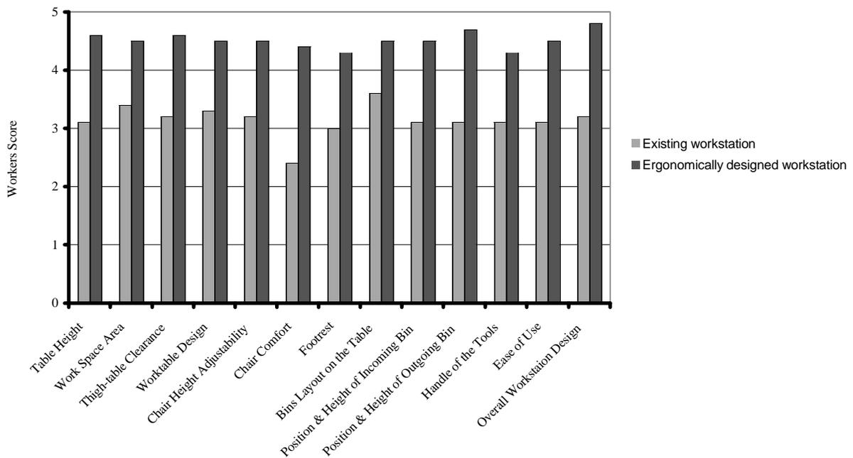
Figure 6. Operator satisfaction with design attributes on two workstations
