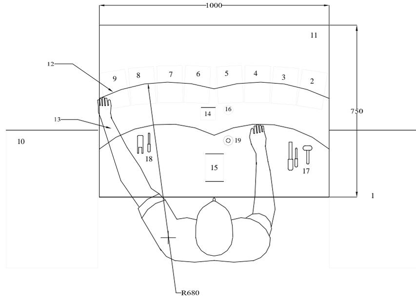
Legend: 1. Incoming bin (600x400); 2. Arc chutes bin (140x110); 3. Terminal clamp bin; 4. Tripping lever bin; 5. Cover parts bin; 6. Handle springs and long screws bin; 7. Handle and handle base bin; 8. Line terminal bin; 9. 3-pole body bin; 10. Outgoing bin (600x400); 11. Assembly table; 12. Maximum reach; 13. Normal reach; 14. Fixture; 15. Assembly area; 16. Grease container; 17. Tool area 1; 18. Tool area 2; 19. Power screwdriver.
