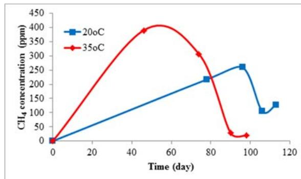
Figure 3c. Methane concentrations in the biogas produced from tomatoes at 20°C and 35°C.
