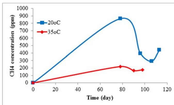
**Figure 3d.** Methane concentration in the biogas produced from orange peels at 20°C and 35°C.
