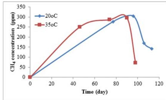
Figure 3a. Methane concentration in biogas produced from zucchini at 20°C and 35°C.
