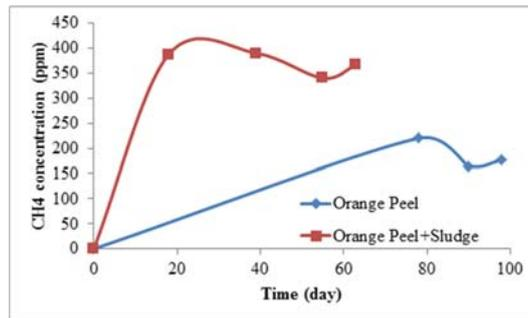
Figure 4-c. Methane gas concentration in the biogas produced from orange peels with and without sludge (T = 35°C).
