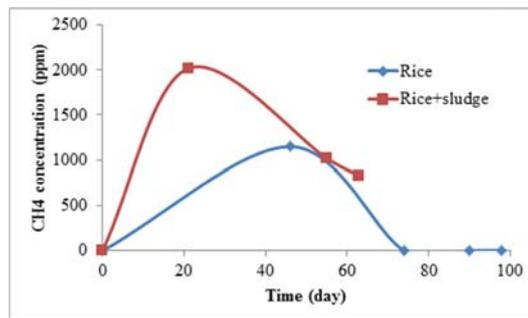
Figure 4d. Methane gas concentration in the biogas produced from rice with and without sludge (T = 35°C).
