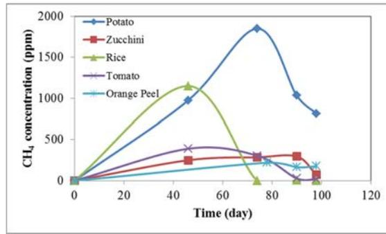
Figure 2. Methane concentration in the biogas produced from the various solid wastes at 35°C.
