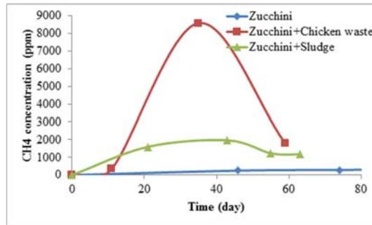
Figure 4-a. Methane gas concentration in the biogas produced from zucchini in the presence of sludge, and chicken dung as an inoculum 35°C.
