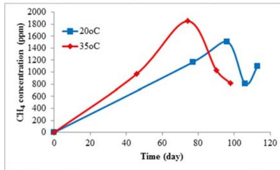
Figure 3b. Methane concentration in the biogas produced from potato at 20°C and 35°C.
