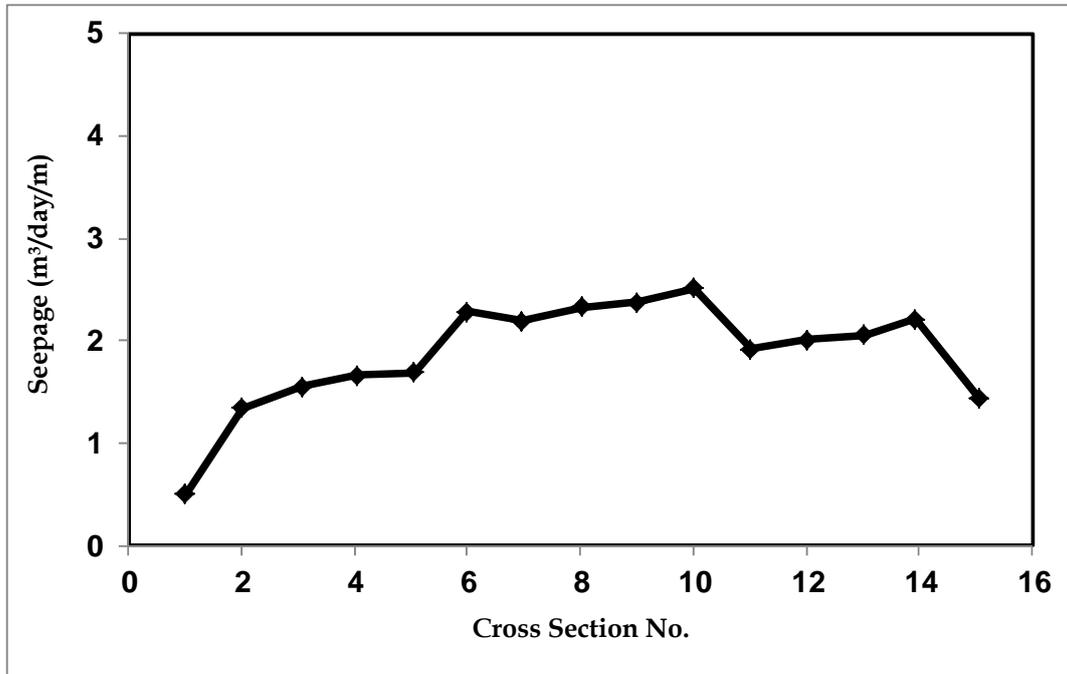
Figure 8. The seepage modeling results of the design case of Al-Fulaij dam.
