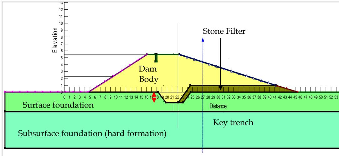
Figure 7. Design case of the dam as modeled in the program (SEEP/W 2007).
