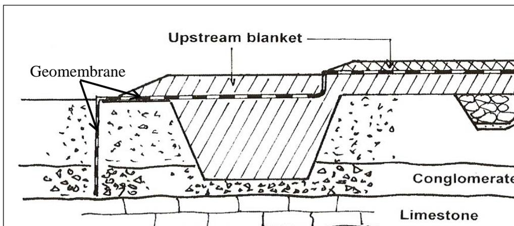
Figure 12. Dam with geomembrane.
