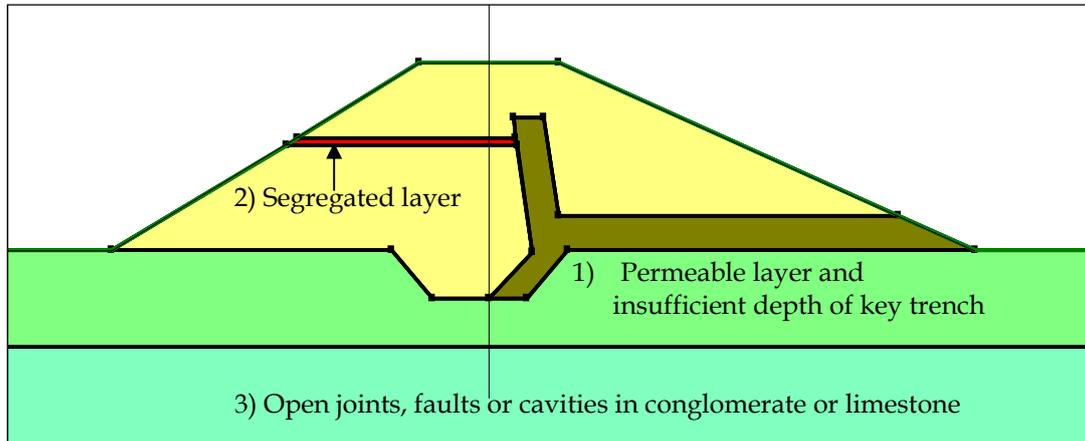
Figure 6. Possible causes of seepage.
