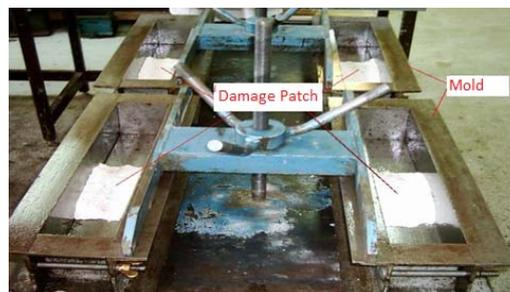
c) Placing the white cement patch in the prism molds before casting.
