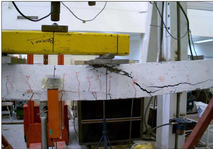
**Figure 12.** Repaired beam after failure.
