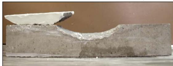
b) Removing the white cement patch.
