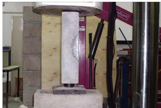
**Figure 3.** Test setup of plain concrete prisms under axial compression.
