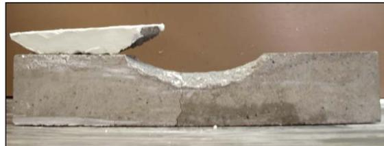
b) Removing the white cement patch.
