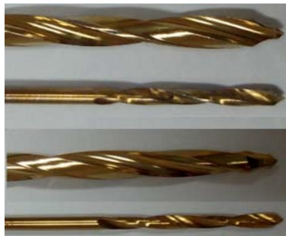
**Figure 2.** Orthopaedic surgical drills used in drilling experiments.
