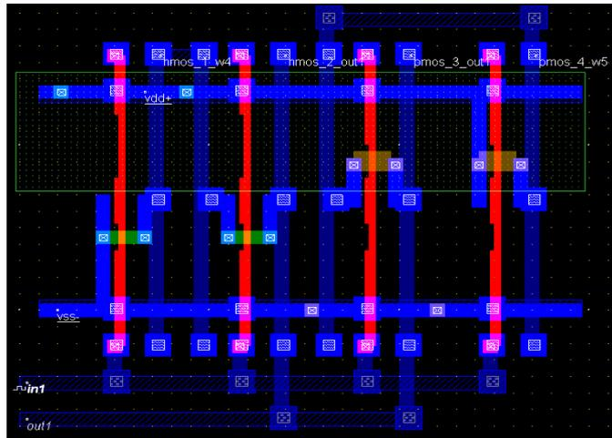
Figure 7. Inverter layout with stack technique in 45nm technology.
