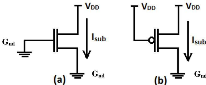
**Figure 2.** Method to measure subthreshold leakage current through (a) NMOS transistor, and (b) PMOS transistor.
