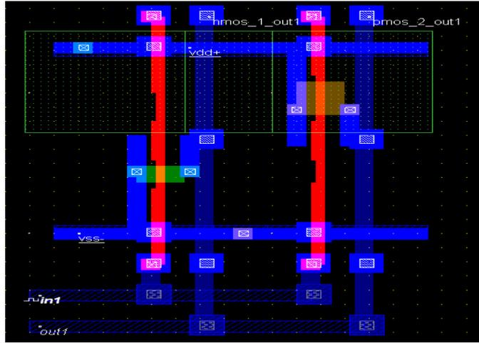
Figure 6. Layout of conventional CMOS Inverter 45nm technology.
