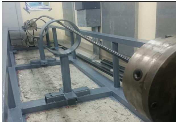
Figure 4. Large deflection of the 1" diameter drill pipe at rotational speed close to its resonance.
