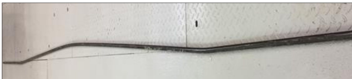
Figure 6. Yielding of 1" diameter drillstring due to operating at 94% critical speed.
