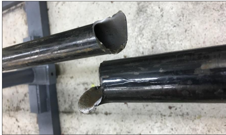
Figure 7. Fatigue failure of 1" diameter drillstring.
