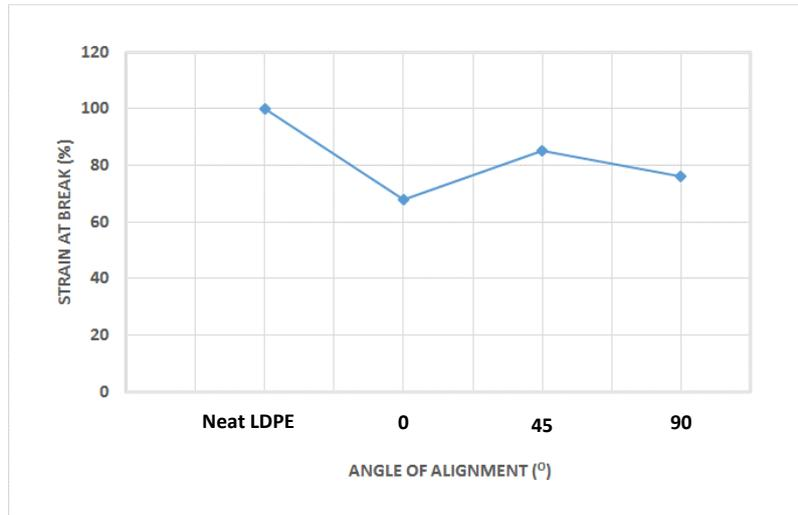
**Figure 4.** Strain at break of the tested bio-composites sheets.
