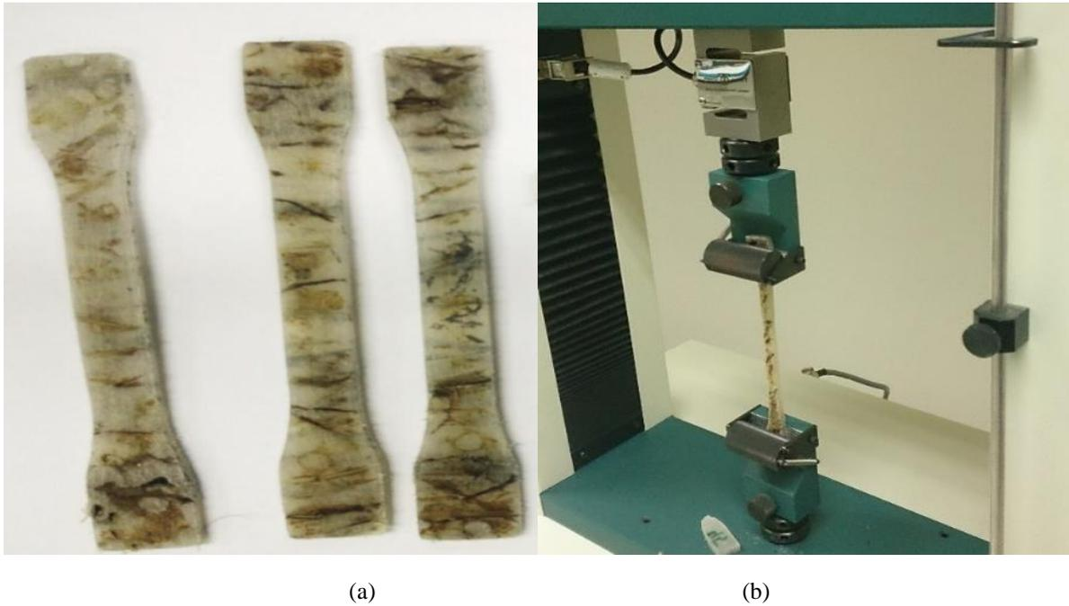
**Figure 2.** Tensile testing procedure ( $\theta = 90^\circ$ ); (a) specimen, and (b) testing setup.
