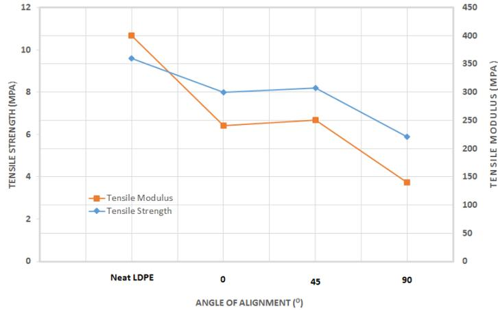
**Figure 3.** Tensile strength (left) and Tensile Modulus (right) of the tested bio-composites sheets.
