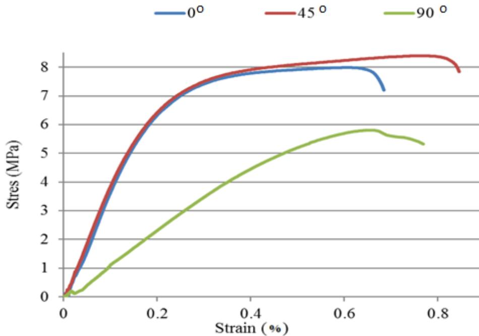
**Figure 5.** Stress-Strain curves in tension of tested specimens.
