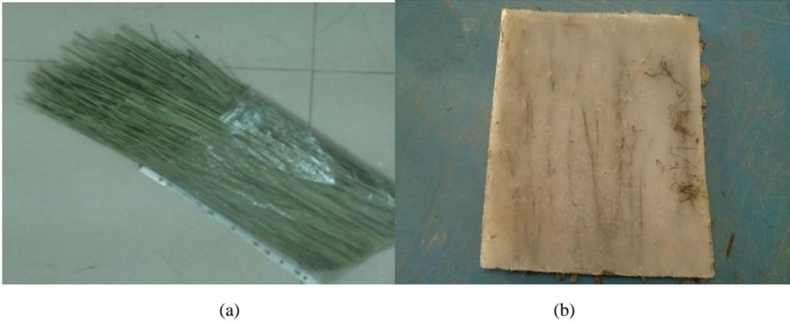
**Figure 1.** Manually extracted date palm fronds fibers; (a) raw, and (b) encapsulated.
