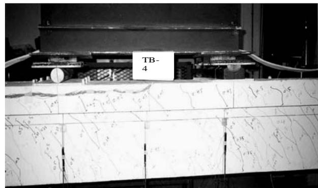
Figure 32. Crack development (TB4)
