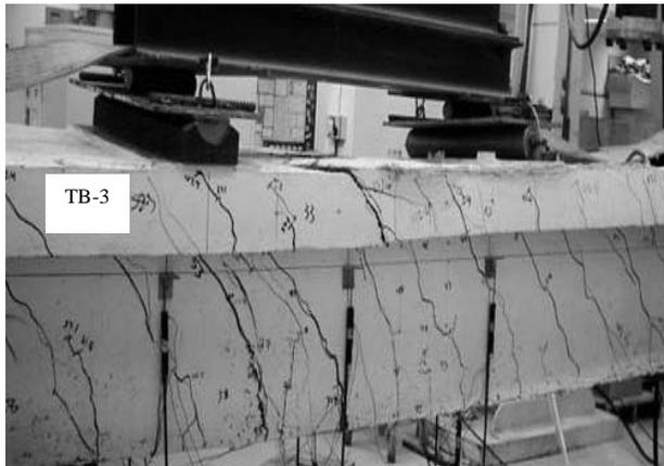
Figure 26. Crack development (TB3)
