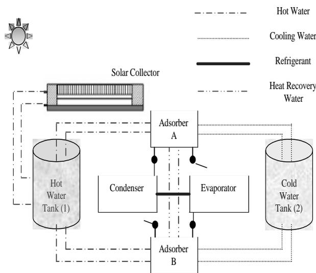
**Figure 8. Solar powered continuous (two beds) adsorption air-conditioning system (Yong and Sumathy, 2004)**
