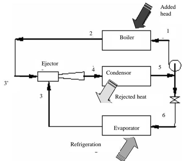
Figure 12-b. Schematic diagram of ejector cycle
