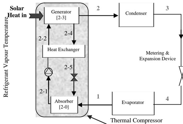
Figure 5-b Schematic diagram absorption refrigeration cycle (single effect)
