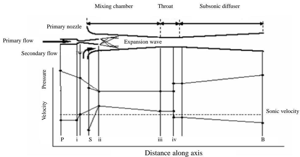
Figure 11. Typical steam ejector and flow characteristic in the ejector (Chunnanod and Aphornratana, 2003)
