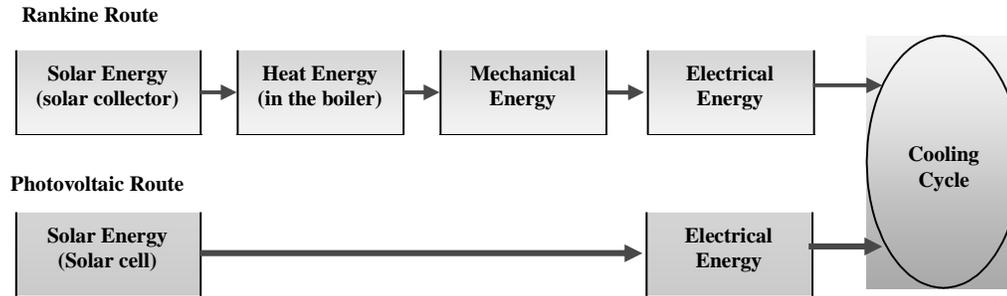
Figure 4. Schematic diagram of Rankine cycle and photovoltaic cycle routes
