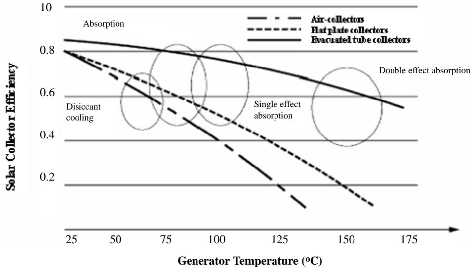
Figure 10. Collector efficiency versus driving heat temperature for various sorption refrigeration systems (Henning, 2000)
