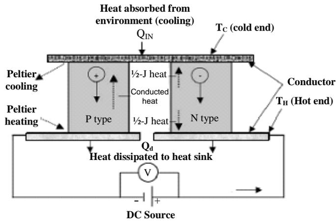
Figure 13-a. Schematic of thermo-electric module operation (Cooling mode), Riffat and Ma, 2003)
