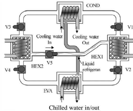
Figure 9-b. Schematic of mass recovery absorption refrigeration cycle, second made (Alam, 2004)
