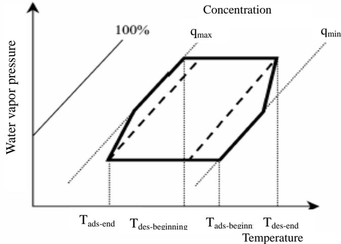
Figure 9-a. PTX diagram for mass recovery cycle
