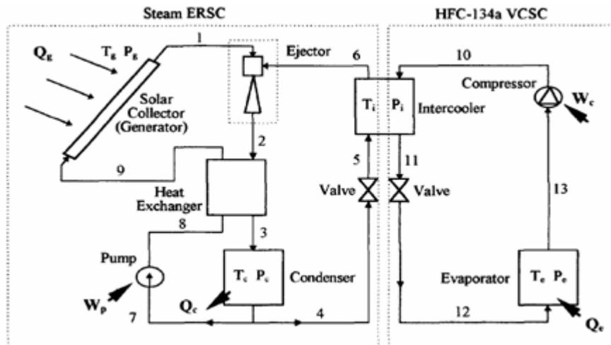
Figure 15. Schematic diagram of a solar-powered combined ejector-vapour compression cycle (Sun, 1997)
