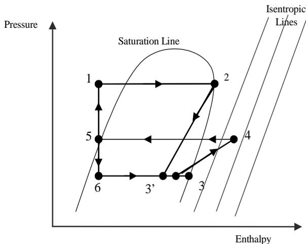
Figure 12-a. P-H diagram of ejector cycle
