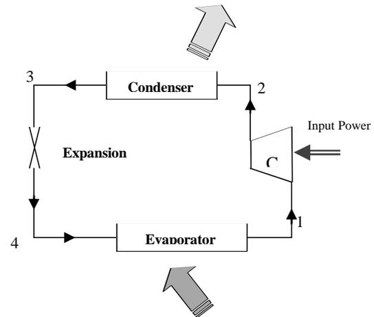
Figure 1-b Schematic diagram for vapour compression cycle
