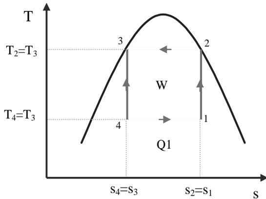
Figure 14-a. Carnot cycle, T-s diagram
