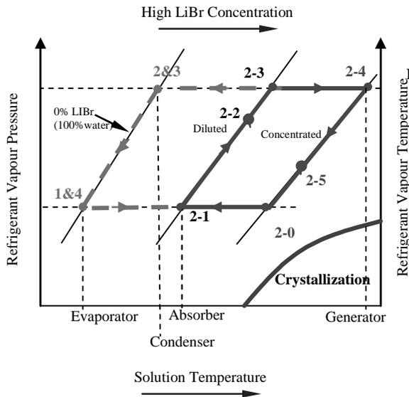
Figure 5-a PTX chart for absorption refrigeration cycle (for single effect)
