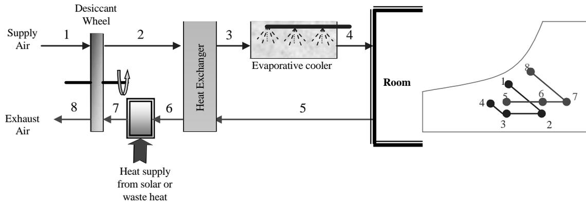
**Figure 6. Desiccant cooling system**
