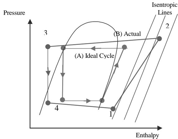
Figure 1-a P-H diagram for vapour compress cycle
