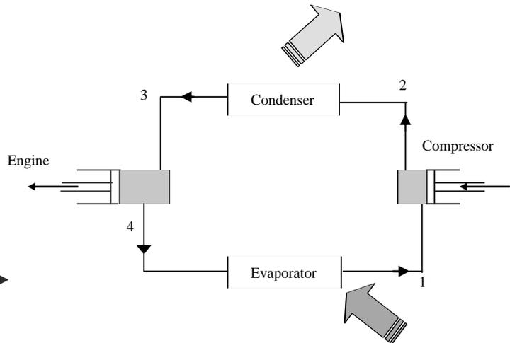
Figure 14-b. Carnot cycle schematic diagram
