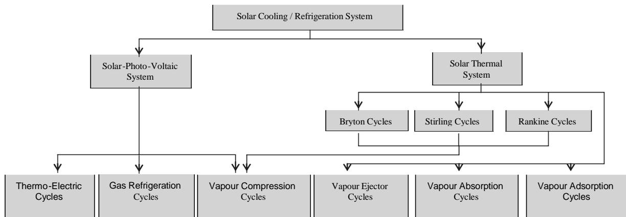
Figure 2. Classification of solar refrigeration cycles
