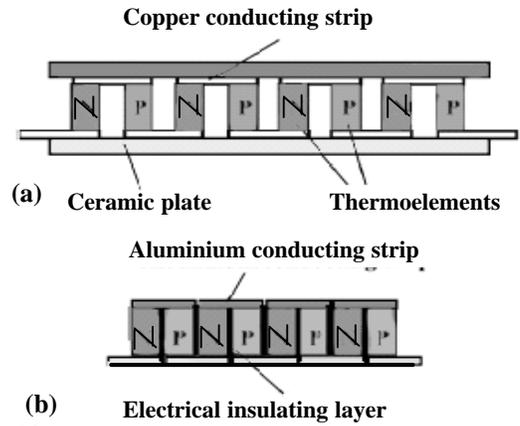
Figure 13-b. Schematic diagram of multicouple thermoelectric modulus
