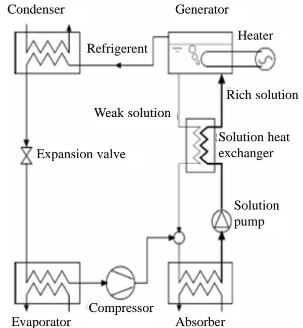
**Figure 16. Schematic diagram of a vapour compression/absorption hybrid cycle. The absorption unit is connected to the compressor exit in series (Mistuhiro *et al.*, 2001)**
