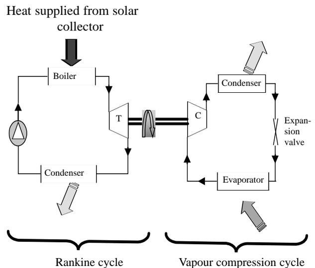
**Figure 3. Schematic diagram of Rankine-vapour compression cooling cycle**
