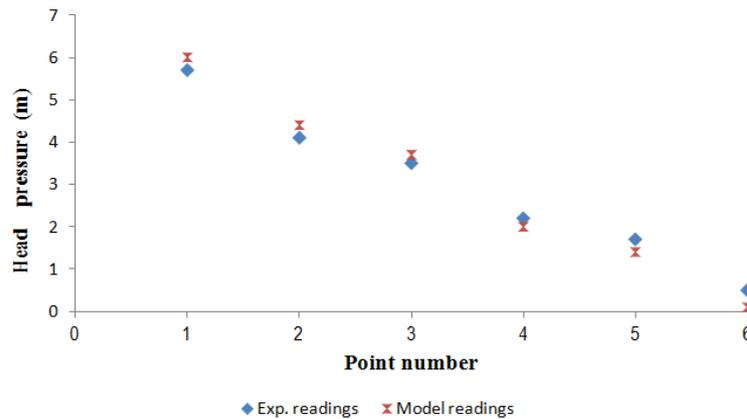
Figure 5. Sample of model calibration H= 6m, L= 20m,  $d_1$  &  $d_2= 5m$ .
