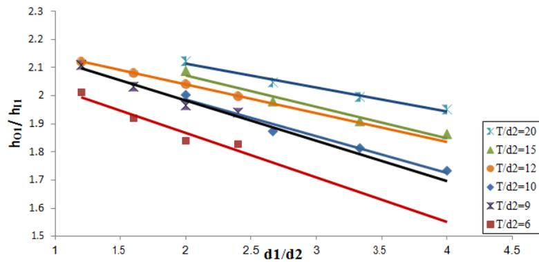
Figure 9. Design chart for the ratio between the head lost along the outer and the inner faces of U.S sheet pile.
