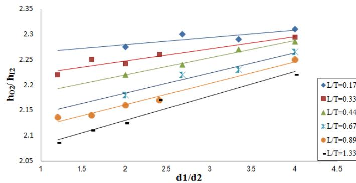
Figure 10. Design chart for the ratio between the head lost along the outer and the inner faces of D.S sheet pile.
