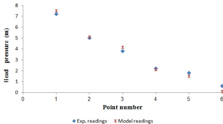
Figure 6. Sample of model verification H= 7.5 m, L= 19 m,  $d_1 = 5m$ ,  $d_2= 2.5m$ .
