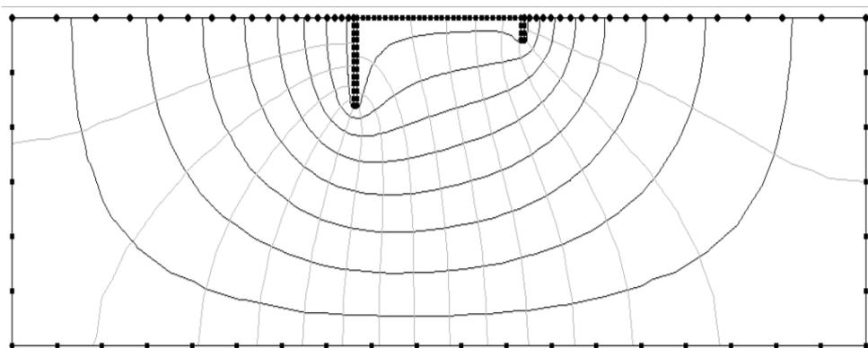
Figure 4. Sample of flow net obtained from SEEP2D (SEEP2D output).
