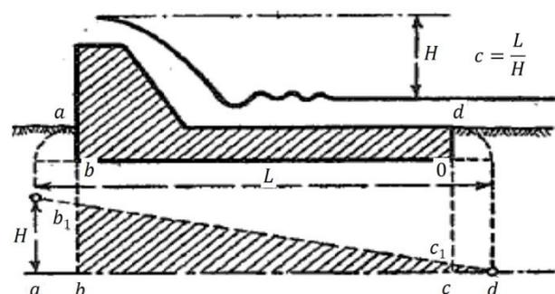
**Figure 1.** Line of creep and hydraulic gradient diagram (after Serge Leliavsky, 1965).
