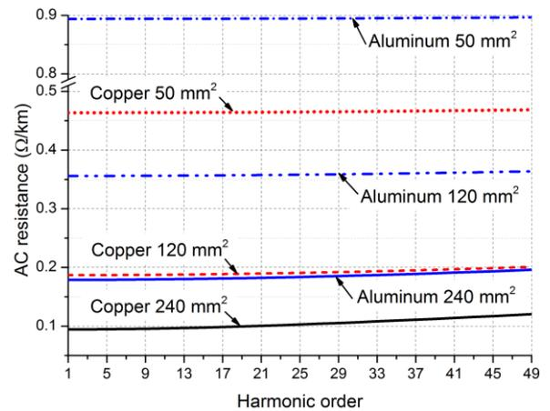
**Figure 7.** Effect of harmonic order on the ac resistance for different sizes and conductor materials of UGC.
