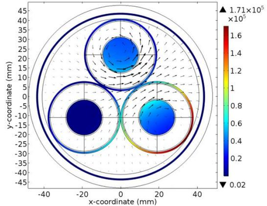
(a) Surface plot of resistive losses ( $\text{W}/\text{m}^3$ ) with proportional arrow direction of magnetic field intensity ( $\text{A}/\text{m}$ ).
