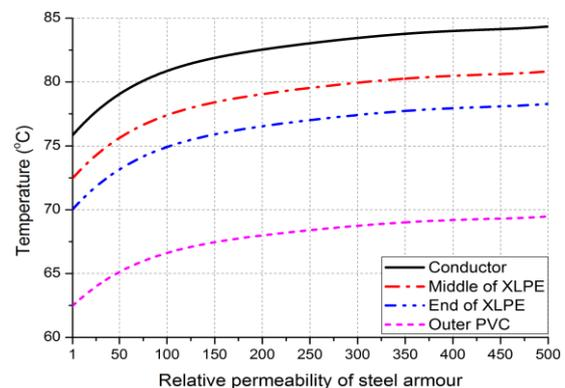
**Figure 5.** Effect of relative permeability of steel armour on the steady-state temperature rise inside different parts of the UGC.
