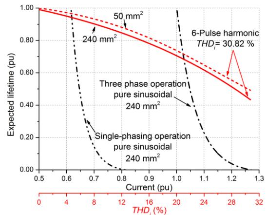
Figure 9. Expected per-unit lifetime of the cable under different operating conditions versus current rating and  $THD_i$ .
