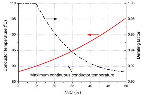
**Figure 10.** Effect of current total harmonic distortion on the conductor temperature and the corresponding derating factor for the 240 mm<sup>2</sup> UGC.
