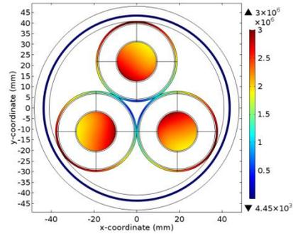
(a) Surface plot of current density ( $A/m^2$ ).
