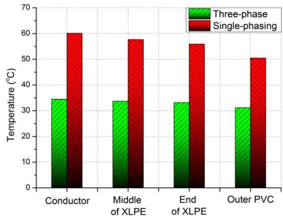
(b) Steady-state temperature at different layers inside the upper core and at the cable surface at half rated current for normal and single-phasing operations.
