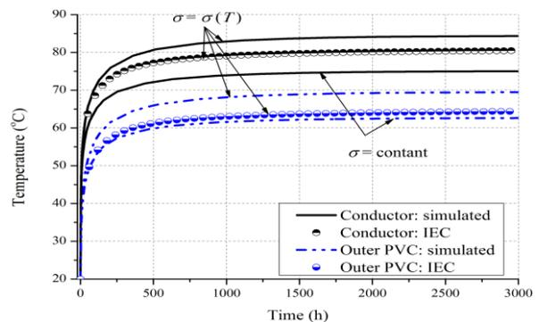
**Figure 4.** Temperature evolution profiles for different points in the core and outer points of PVC jacket until steady-state after 3000 h of simulation compared with the IEC standard calculation.
