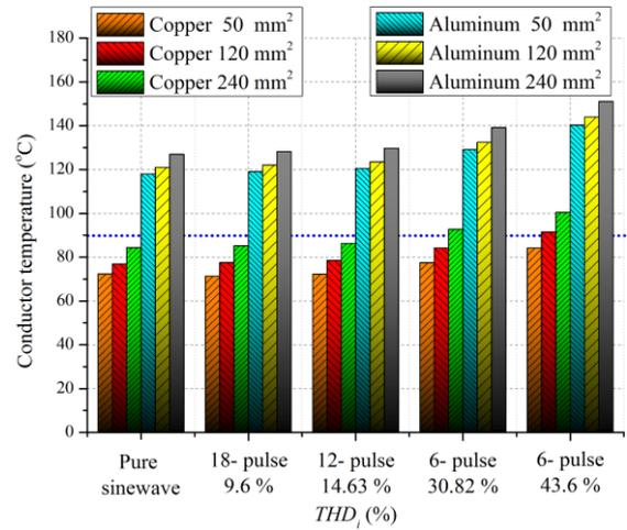
Figure 8. Effect of current total harmonic distortion of the steady-state conductor temperature rises for different sizes and UGC materials
