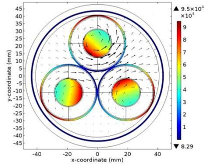
(b) Surface plot of resistive losses ( $W/m^3$ ) with proportional arrow direction of magnetic field intensity ( $A/m$ ).
