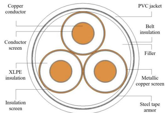
**Figure 1.** A typical 2D cross section of three-phase screened three-core belted underground cable.
