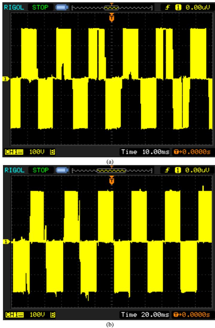
Figure 6. (a) Inverter output voltage (L-L) for  $m=0.96, f=50$  Hz (b) Inverter output (L-L) for  $m=0.48, f=25$  Hz.
